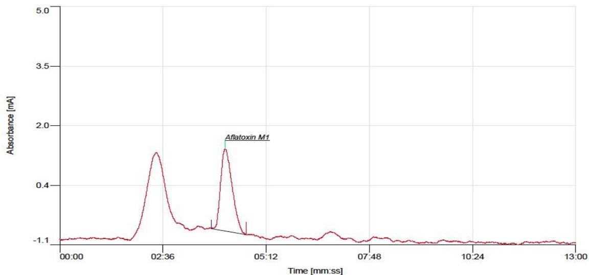
**Fig. 16: Chromatogram of Aflatoxin M1 of *Wagashi* sample using HPLC-FD showing positive detection.**
