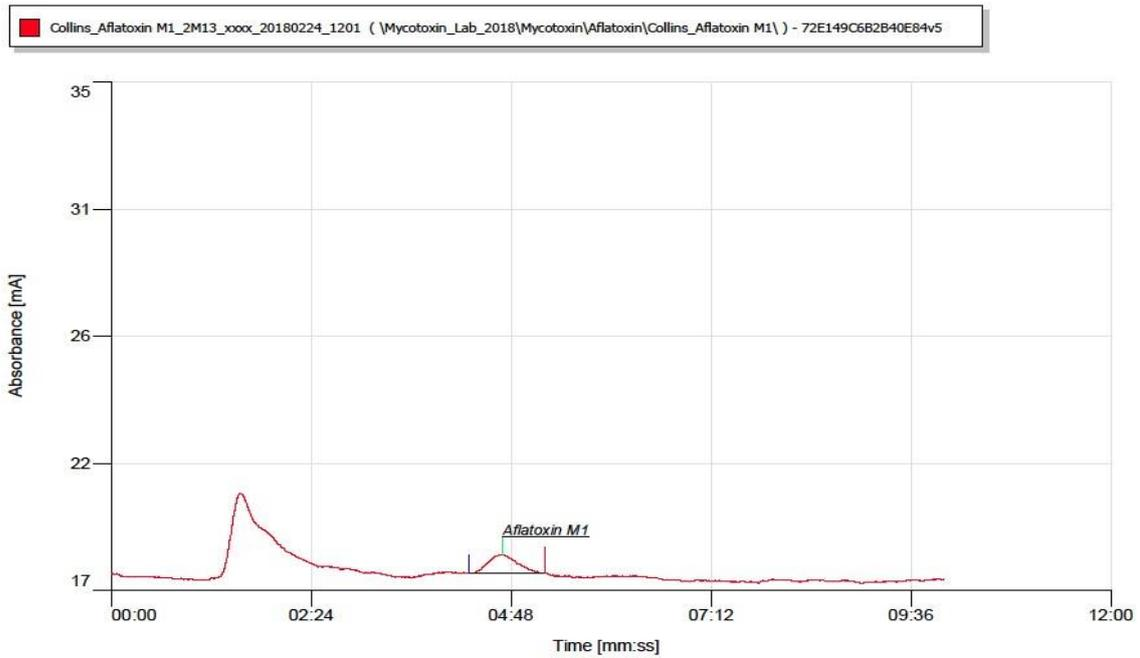
**Fig 10: Chromatogram of Aflatoxin M1 of raw cow milk sample using HPLC coupled with fluorescence detector showing positive detection.**
