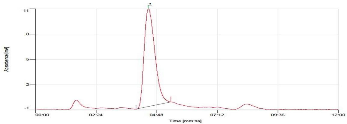
**Fig. 9: Chromatogram of Aflatoxin M1 standard using HPLC coupled with fluorescence detector and PBPB as post column derivatization agent.**
