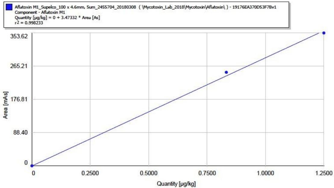
**Fig.8: Aflatoxin M1 standard calibration curve**
