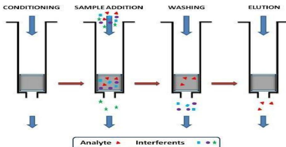
Fig. 5: Schematic diagram of SPE clean-up procedure. (Lucci *et al.*, 2012)
