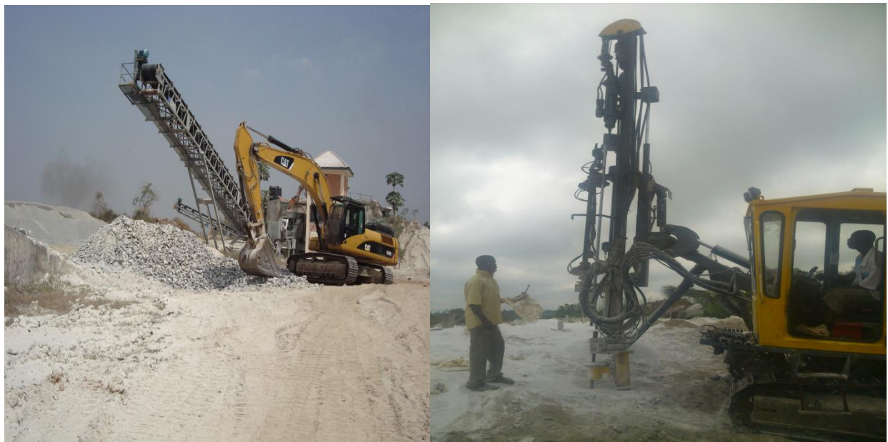
Plate 1. A Pull Loader Filling a Crusher with Blasted Stone Products and Mobile Ridge, Britak Quarry site, Bepotrim.
