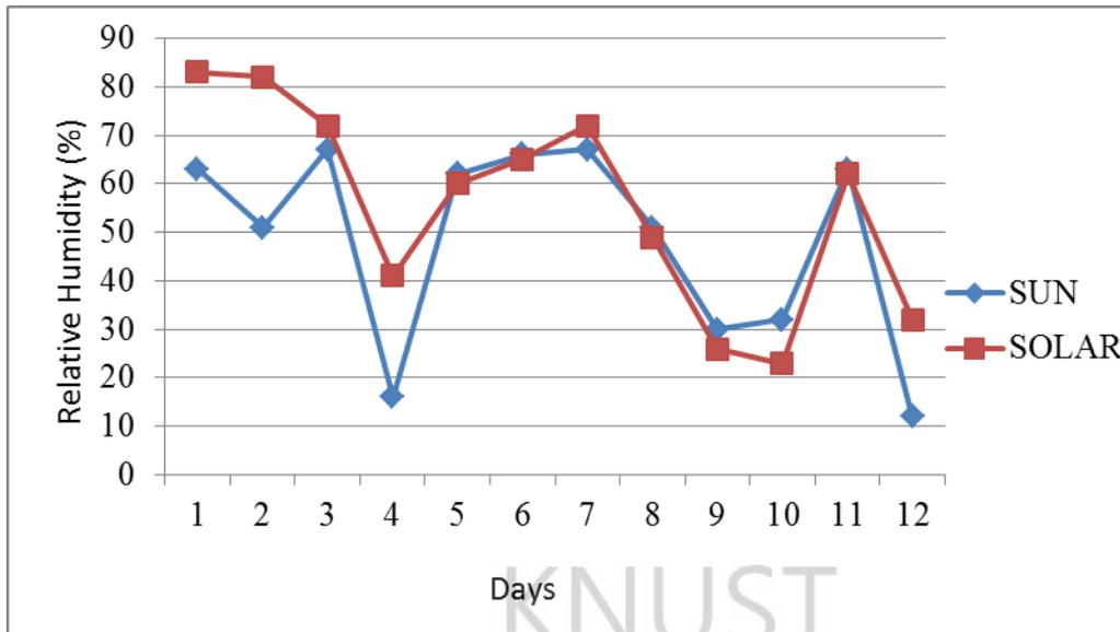
**Figure 4.2. RELATIVE HUMIDITY IN DRYERS DURING DRYING OF PEPPER**
