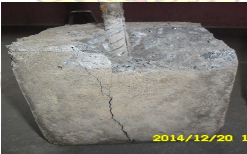
Fig 3: Longitudinal splitting of concrete
