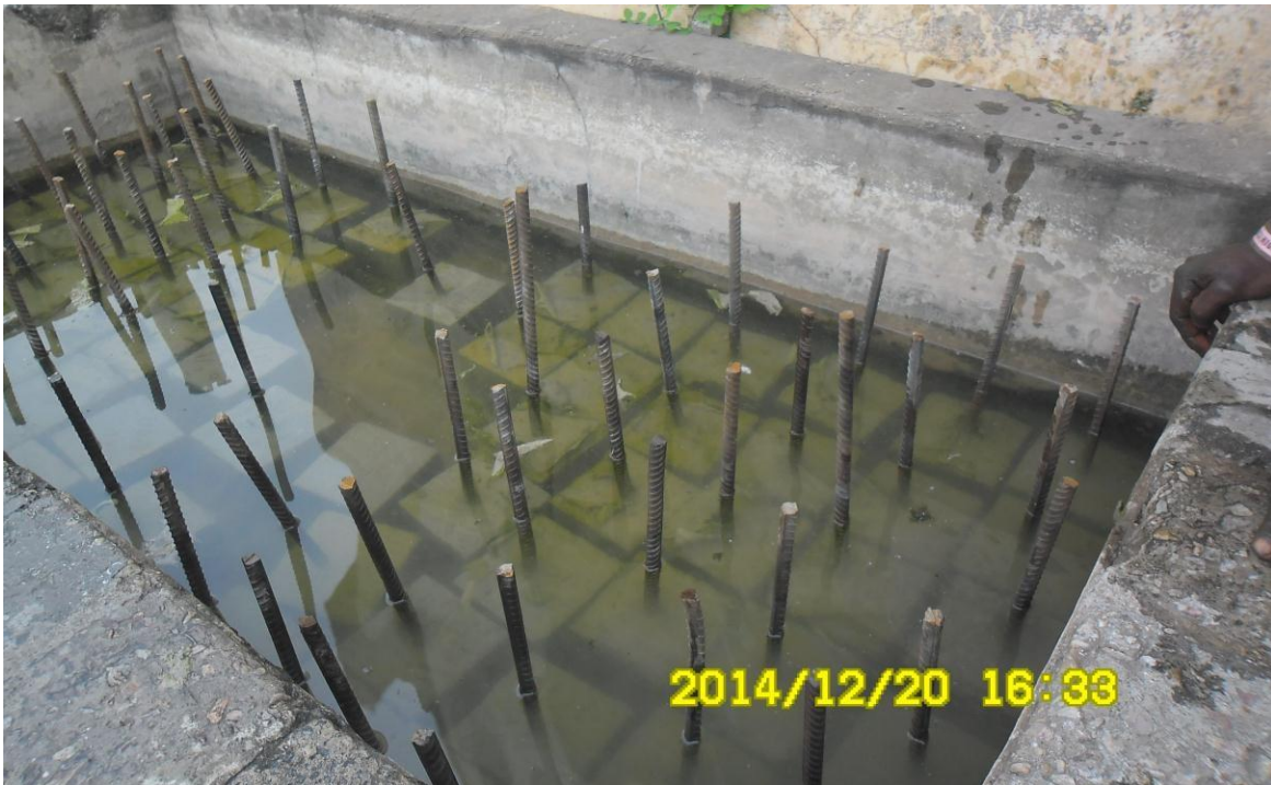
Fig 3.5: Curing of specimen
