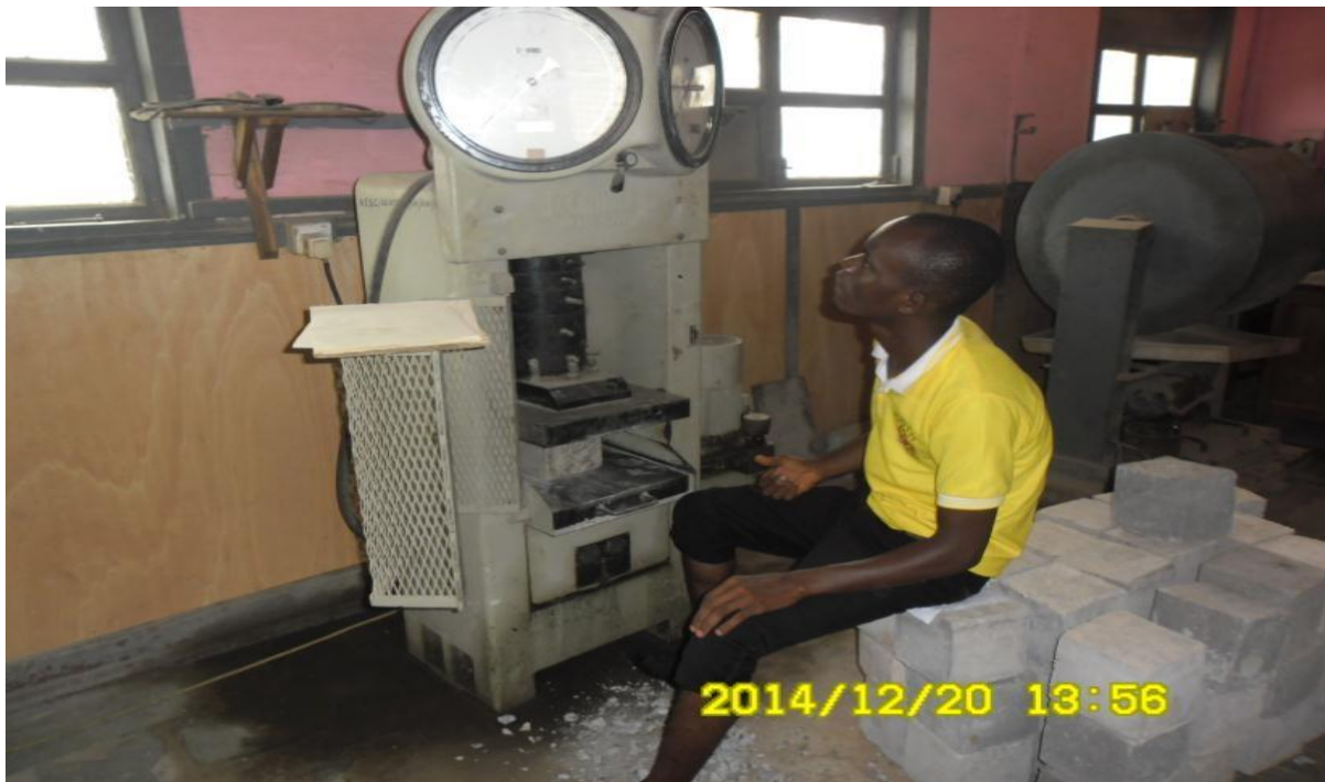
Fig 6: Compressive Strength Test
