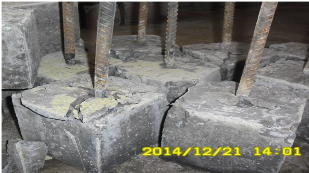
Fig 4: Pull out of rebar
