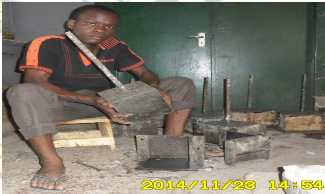
Fig 3.4: Removal of cubes from mould after 24 hours
