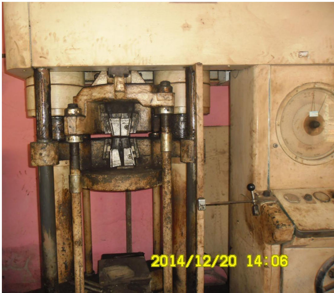
Fig 3.9: Set up for Pull out Test
