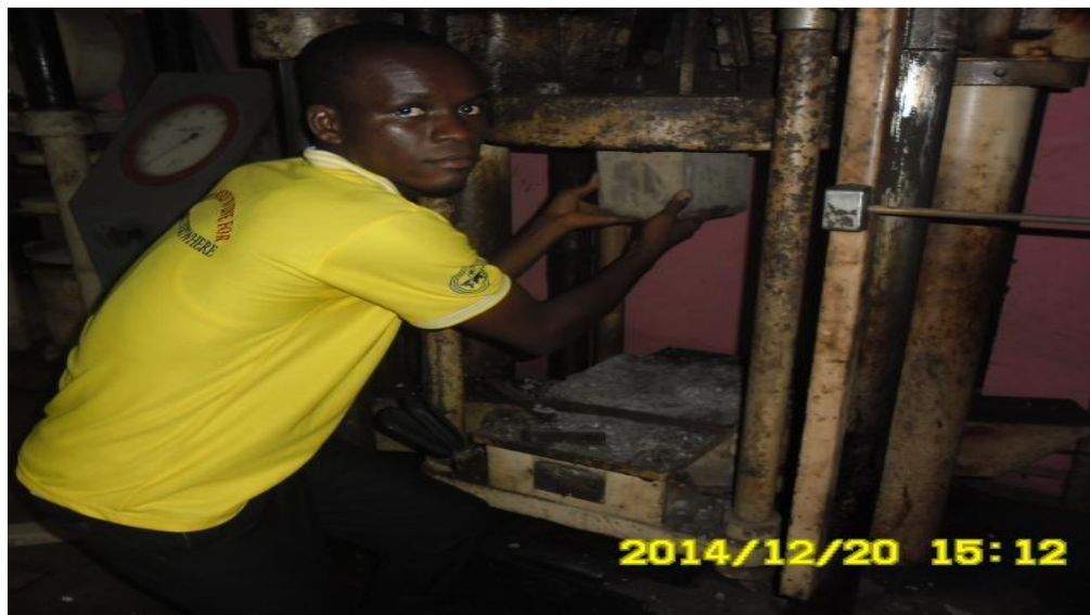
Fig 2: Inserting specimen into Pullout test apparatus
