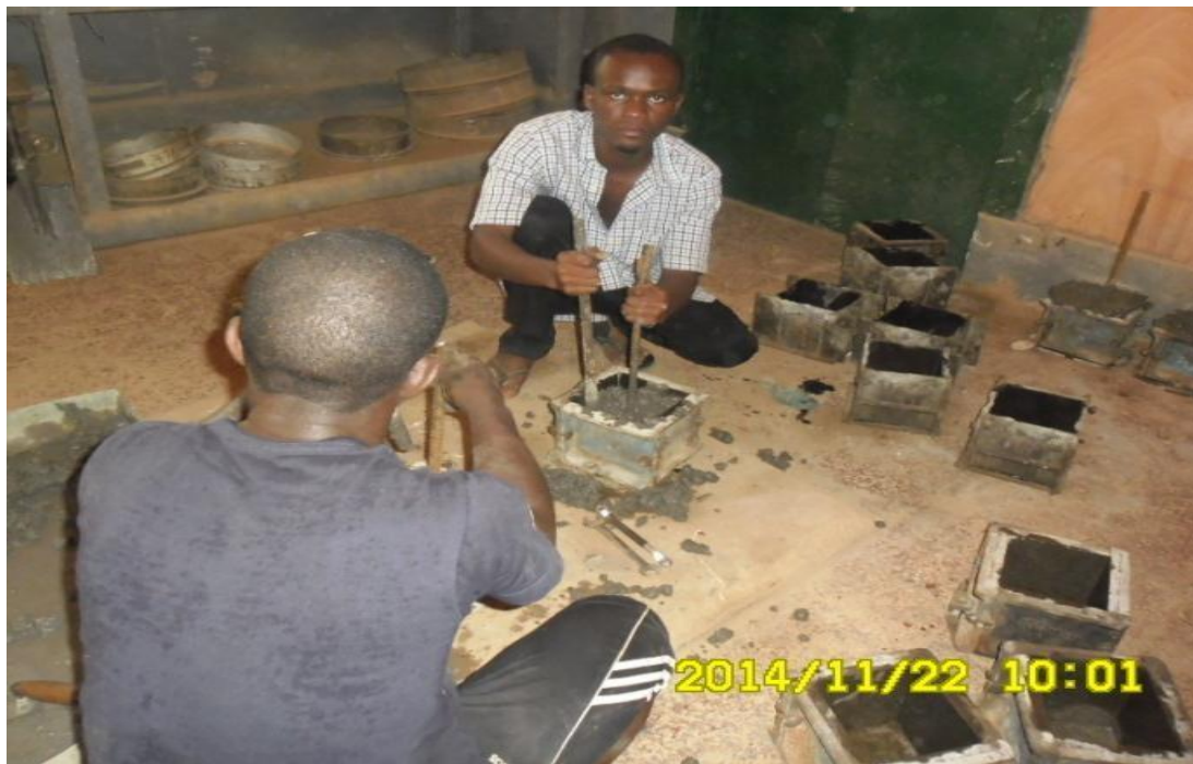
Fig 3.3: Casting of concrete cubes
