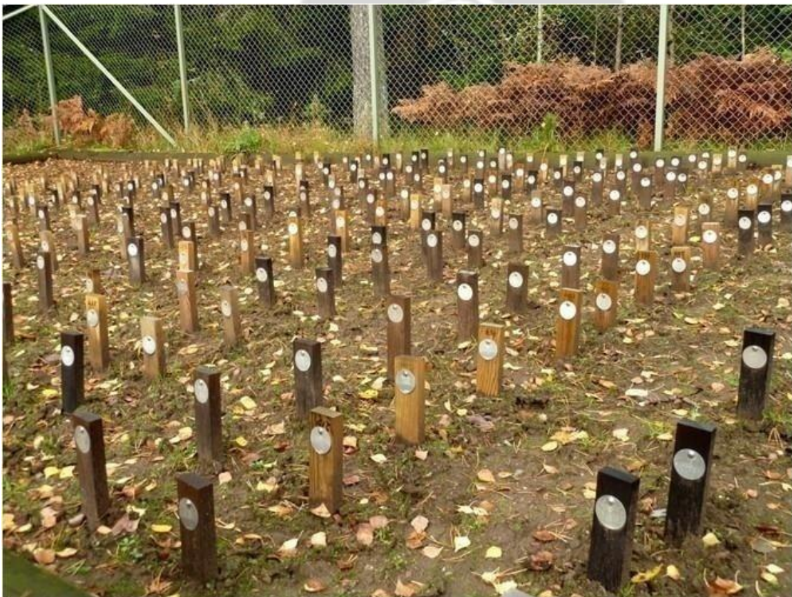
Figure 3.4. B. aethiopum stakes inserted in the test field for natural durability determination at FRNR (KNUST) Experimental Farm
