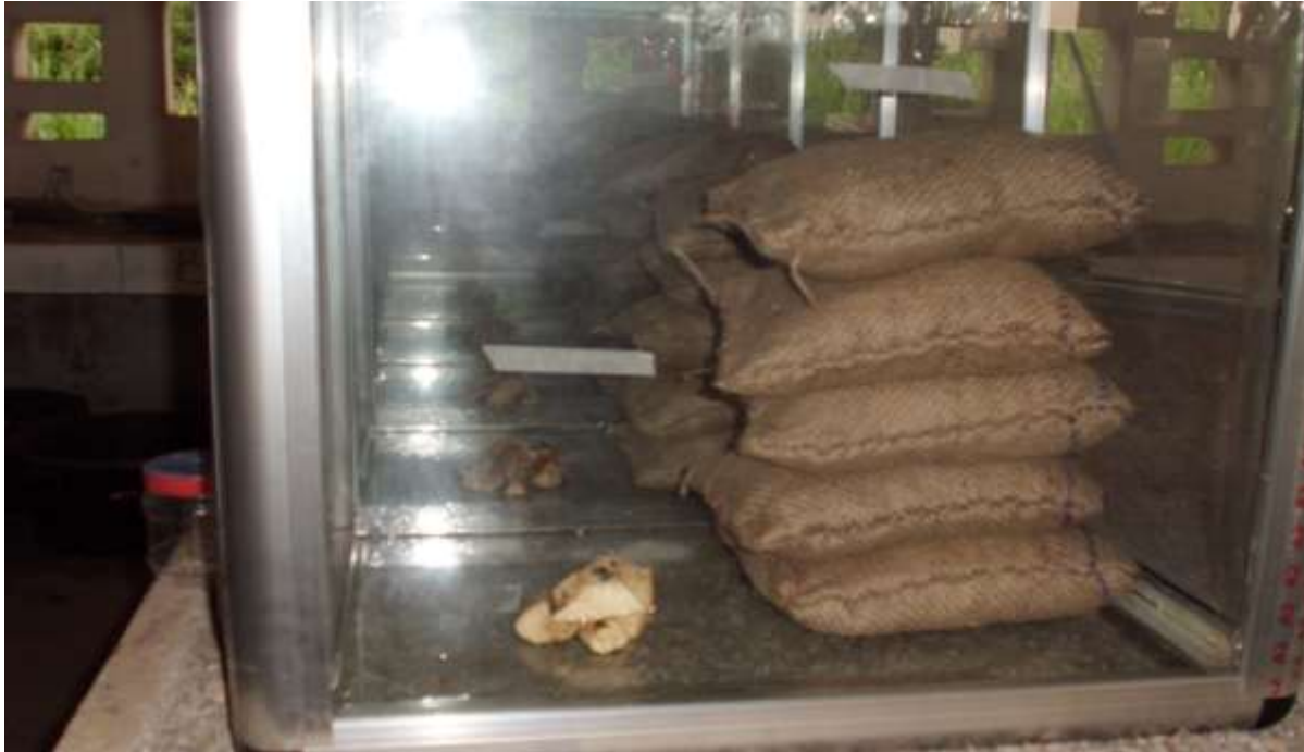
Plate 6: Set-up to determine efficacy of insecticidal cassava bait in the control of A. fasciculatus on bagged cocoa beans
