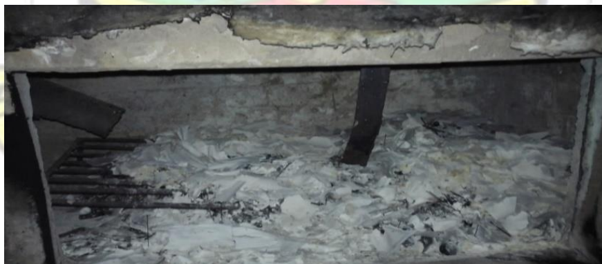
Figure 4.20: Residue (ash) from incineration containing burnt needles and blades. This practise is consistent with guidelines by Ghana's (MLGRD and EPA, 2002) which states that ash produced from the incineration process should be landfilled. Heavy metal waste, by (WHO, 2014) guidelines, must be sent back to the original suppliers
