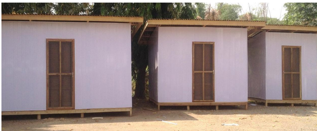
Plate 8: Experimental Rooms (34 m 3 , 19 m 3 and 8.5 m 3 . From Left to Right)
