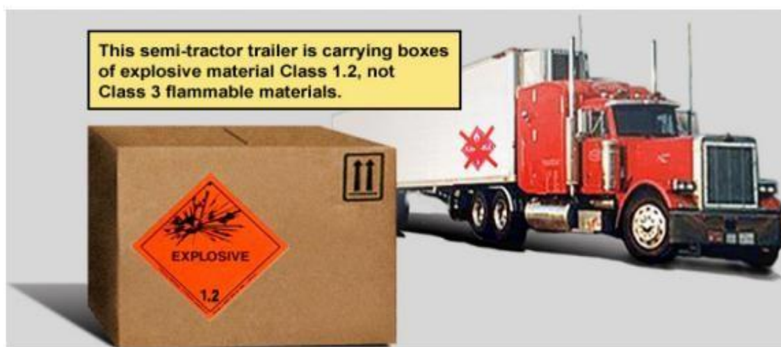
Plate 2.9.1: Placards used in hazardous materials transportation.
