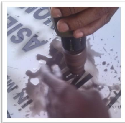
Plate 29: Perforating holes on the text Plate 30: Applying silicone and pieced text on the base
