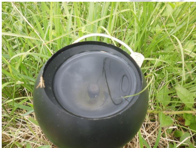
Figure 3.3: Image showing a clogged DOG observed during field visit.
