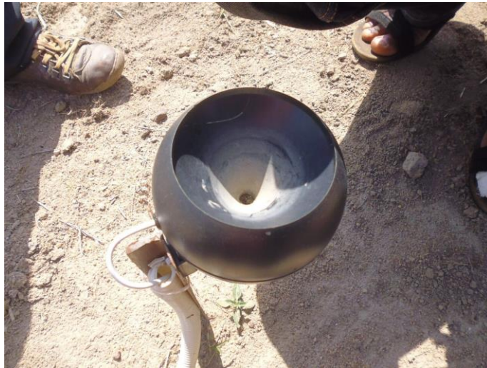
Figure 3.4: Image showing dust particles in the collector of DOG observed field visit.
