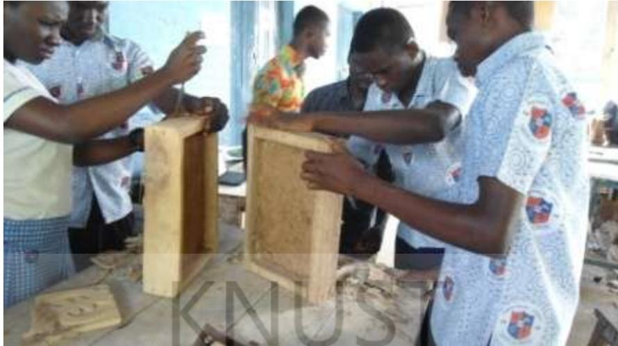
**Plate 3.29 A group of students using a chisels to remove a mould**
