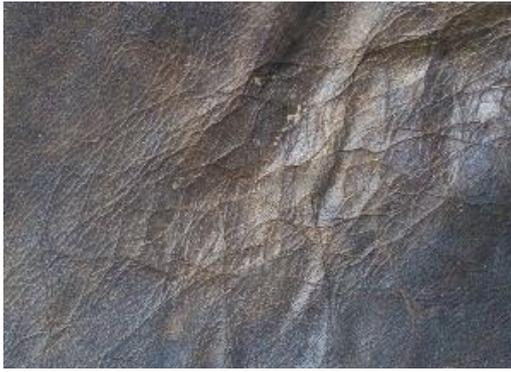
*Plate 40- Wrinkle marks defect*
