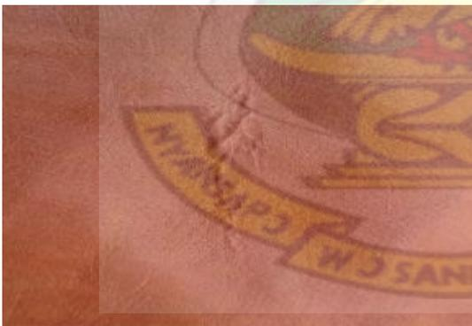
*Plate 36- Grain losing defect*
