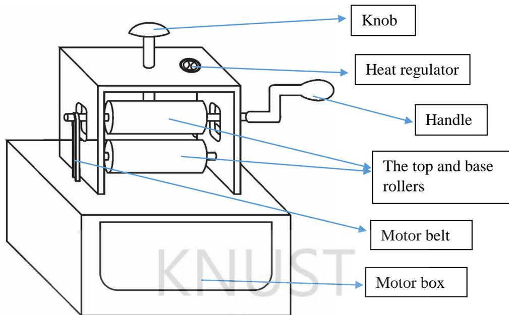
**Figure 9- Design for texturing device**
