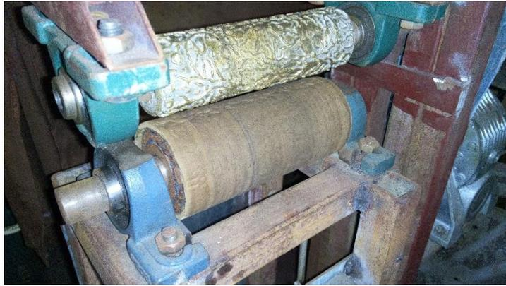
*Plate 17- Based roller wrapped with carbon rubber*
