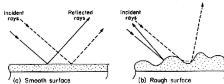
**Figure 4- Light reflection from a smooth and rough surface**
