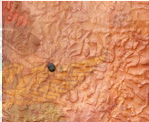
*Plate 86- A hole defect at belly side of the leather.*
