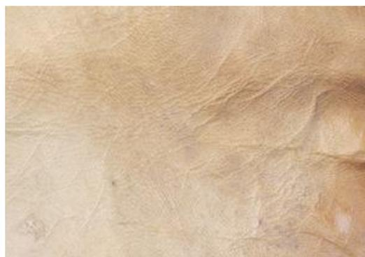
*Plates 25- Wrinkle marks defect*
