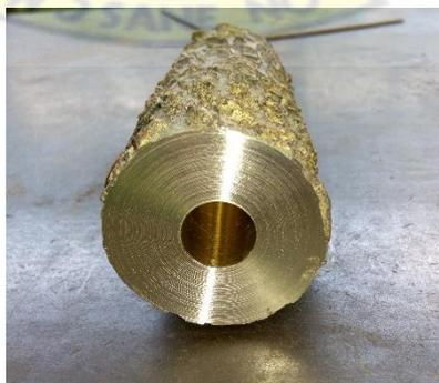
*Plate 9- Meal roller with hole drilled through the center*
