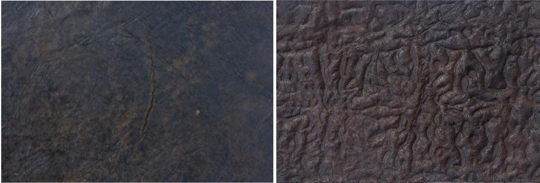
*Plate 98- A grain break at bend side of the leather.*
