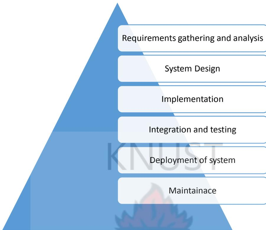
***Figure 5- Sequential phases of Waterfall Model***
