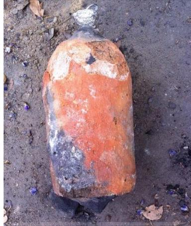
*Plate 7- POP mould with metal cast inside*
