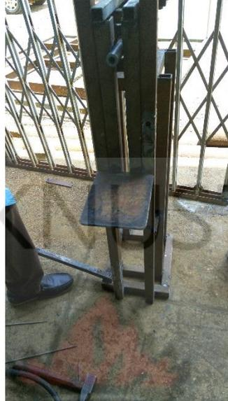
***Plate 13- Motor platform corresponding to one end of the top roller shaft***
