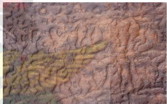
*Plate 93- Mold defects at belly side of the leather.*
