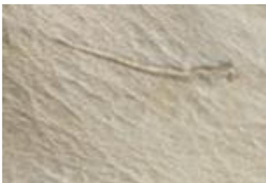
*Plate 24- Cut Defect*
