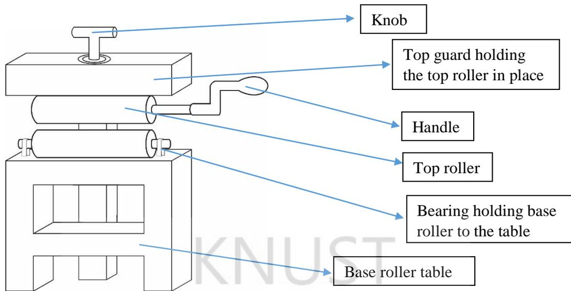
**Figure 10- Design for texturing device**
