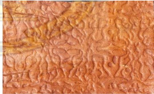
*Plate 78- A mold defect at shoulder side of the leather.*
