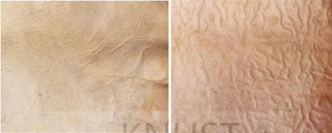
*Plate 73- A wrinkle defect at the belly side of the leather.*
