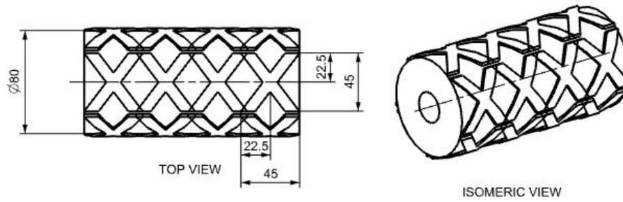
**Figure 15- The top roller in different views**
