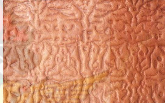
*Plate 77- A patch or an uneven dyeing at the bend side of the leather.*
