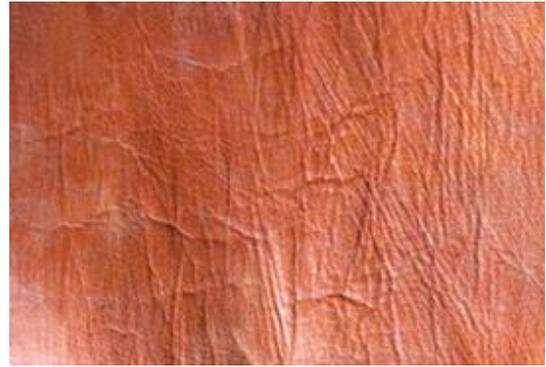
*Plate 33- Wrinkle marks defect*
