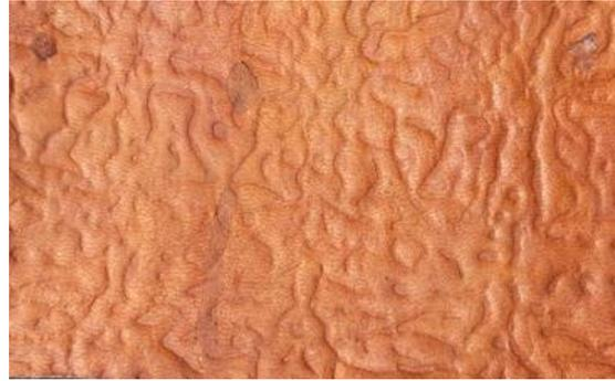
*Plate 76- A grain peelings at the bend side of the leather.*
