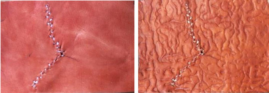
*Plate 79- A stitch patch defect at bend side of the leather.*
