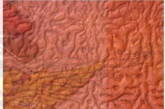
*Plate 83- Scratch marks at bend side of the leather.*
