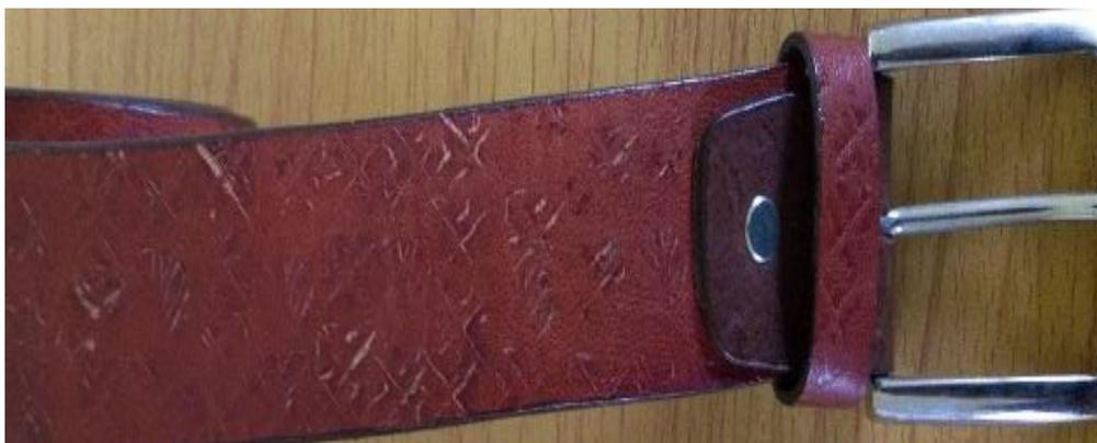
***Plate 53- Stamped leather belt with varying depth***
