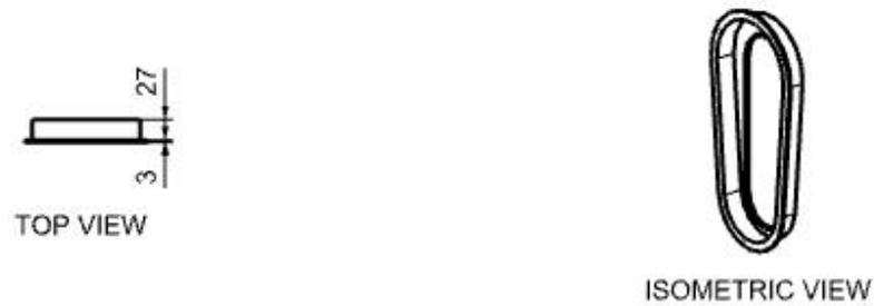
**Figure 18- The sprocket lid in different views**
