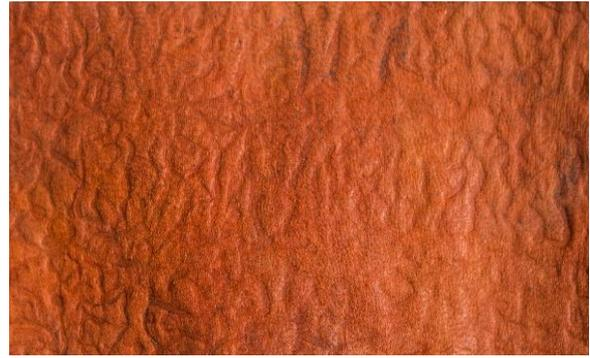
*Plate 82- Wrinkle marks at belly side of the leather.*
