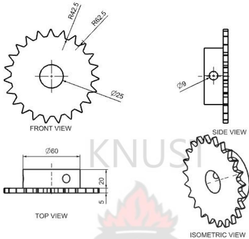
**Figure 17- The sprocket in different views**
