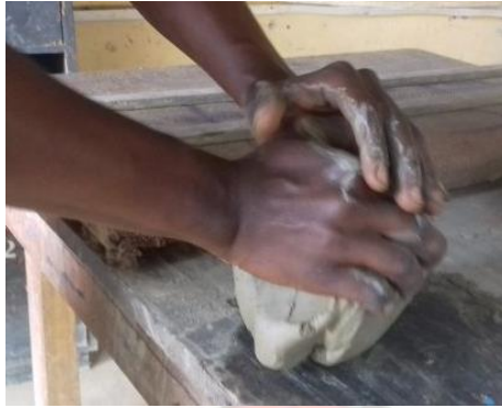
Plate 3.18: Kneading the clay
