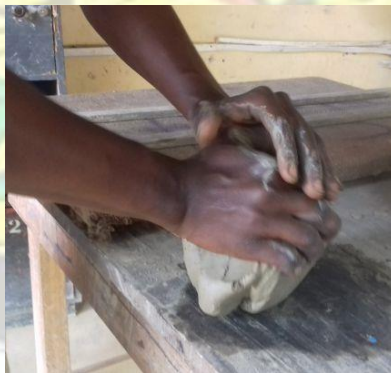
Plate 3.6: Kneading a plastic clay
