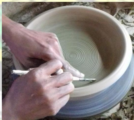
Plate 3.9: Creating the concentric circles in the bowls
