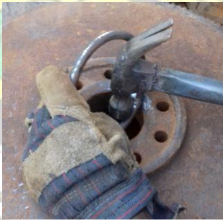
Plate 3.88: Forming the rings
