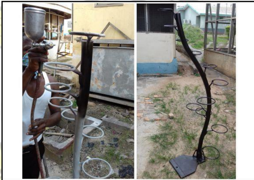
Plate 3.97: Applying the stain
