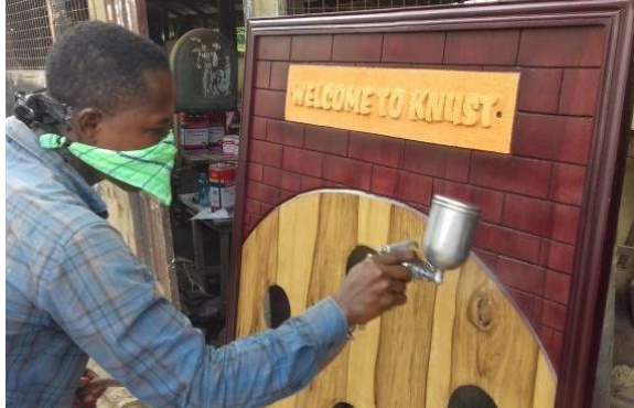
Plate 3.73: Applying lacquer and auto-base clear.
