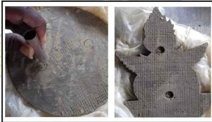
Plate 3.27: 0.8mm depth created at the back of the logos
