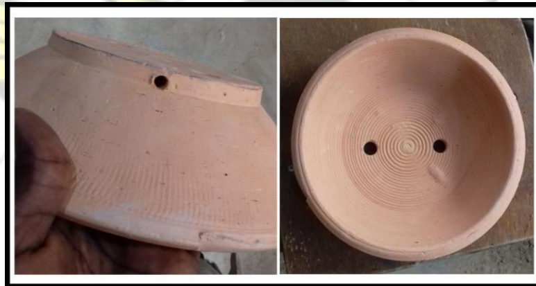
Plate 4.1: the modified asanka bowl showing the foot and center lockers
