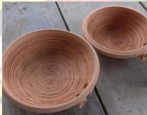
Plate 3.82: The bowls in the bisque state
