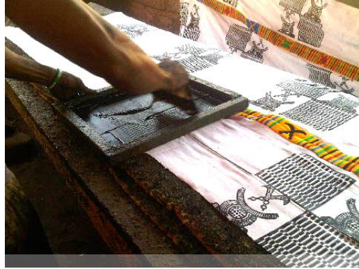
Plate 4.40: Position of the screen on the fabric when printing
