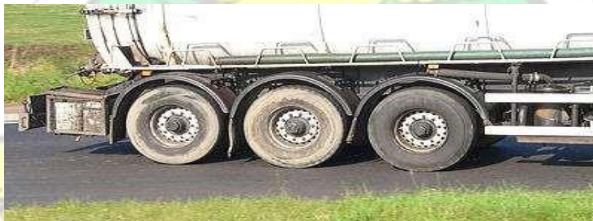
Figure 2.7. HGV trailer with three back axles (Summers, 2000)
