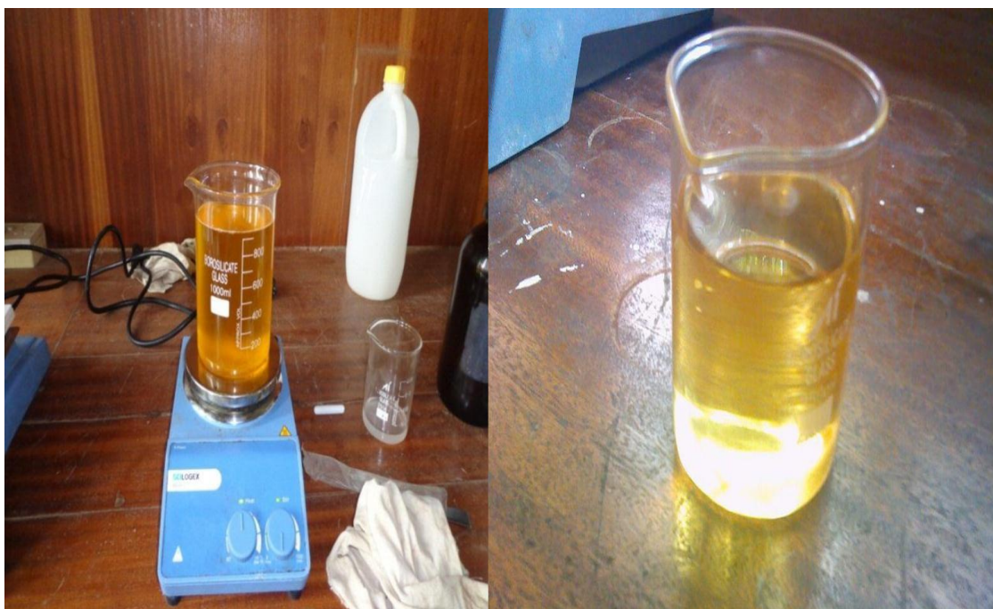
Figure A9 Figure A10 (a) Heating to remove traces of moisture (b) Refined biodiesel
