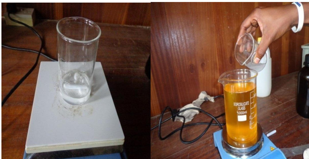
Figure A1 Figure A2 (a) Stirring of Methanol and sodium hydroxide (b) Adding the solution to the oil
