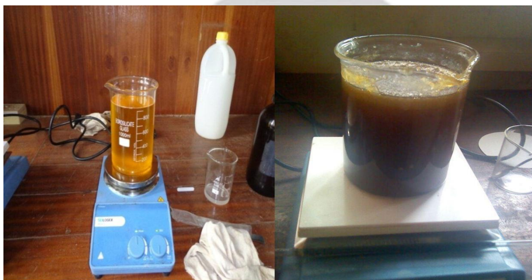
Figure A3 Figure A4 (a) Solution might cake after an hour (b) Sulphuric acid is added at 35°C.
