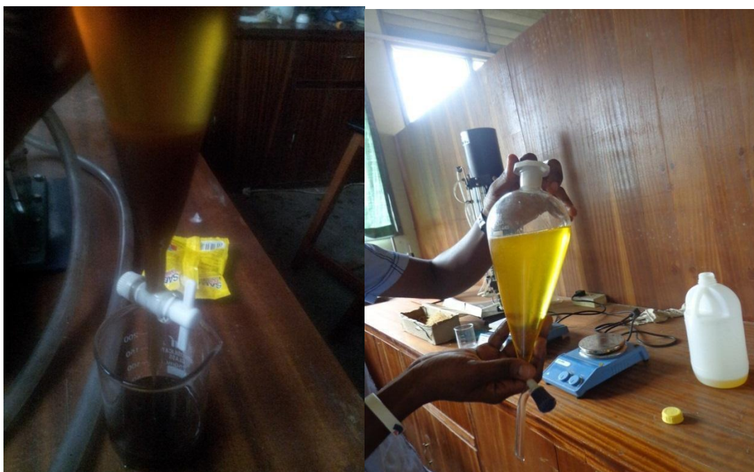
Figure A5 Figure A6 (a) Separation stage (b). Crude biodiesel before washing
