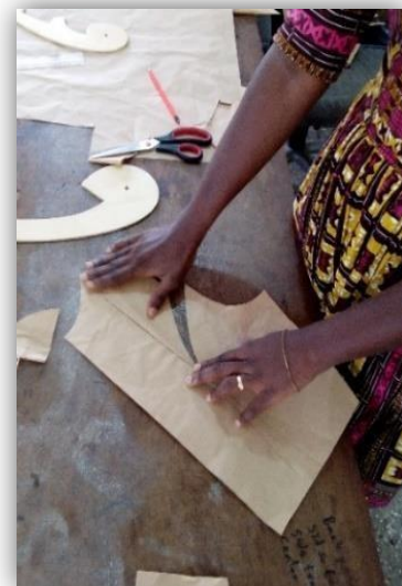
Plate 4.53: Closed shoulder dart opened at armhole
