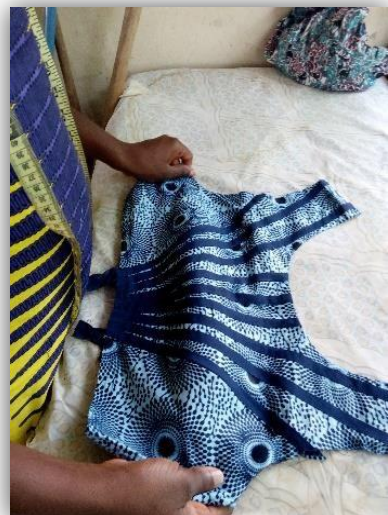
Plate 4.59: Attaching band at waist
