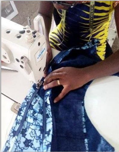
Plate 4.46: Stitching invisible zip at bust
