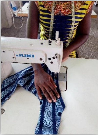
Plate 4.56: Stitching of bias binding
