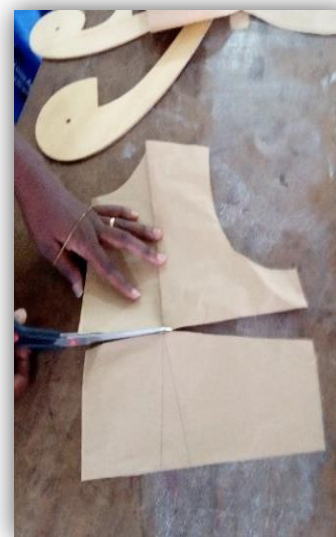
Plate 4.36: Cutting through bodice
