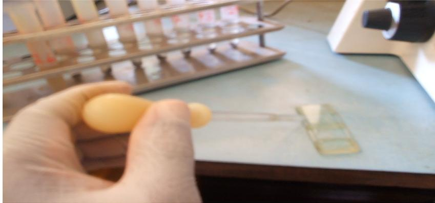
**Fig.16: Filling of McMaster Egg Counting Chamber with prepared samples**
