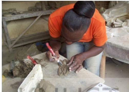
Plate 3.7: Design taken out of mould and trimming
