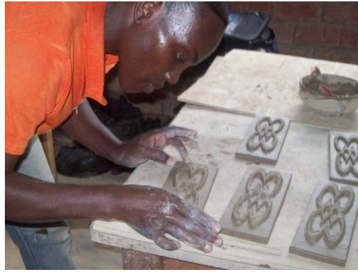
Plate 3.8c: Putting embossed design over slices
