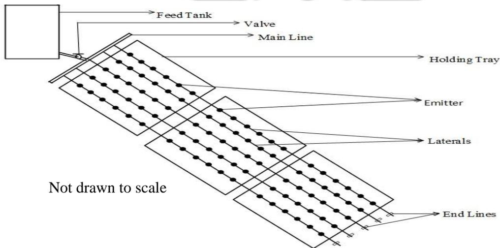
Figure 7 Schematic representation showing laterals and emitters
