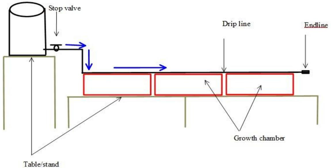
Figure 6 System Flow Chart for one gravity-fed aeroponic unit
