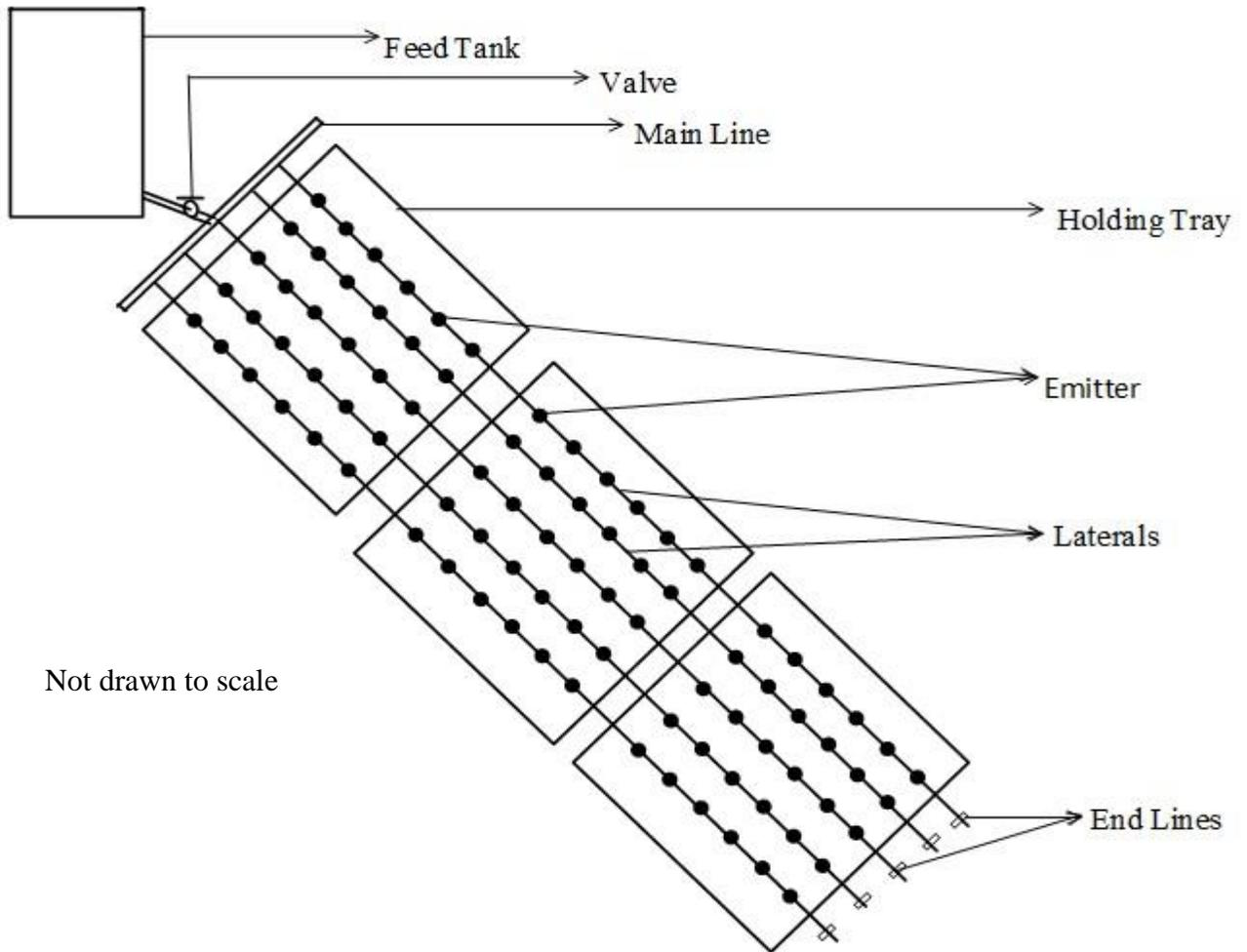
**Plate 3- 7 Schematic representation showing laterals and emitters**
