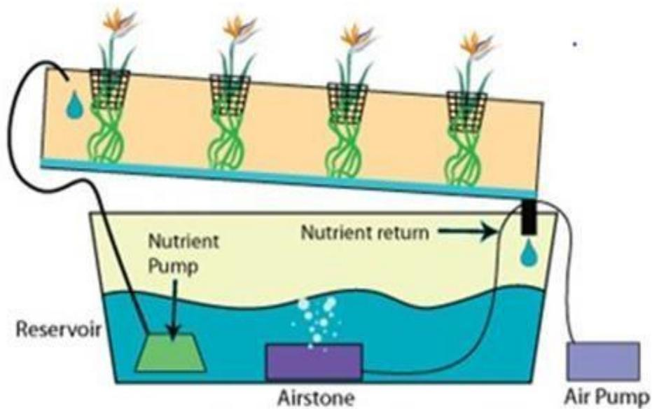
**Plate 2- 1 Schematic representation of the nutrient film technique**
