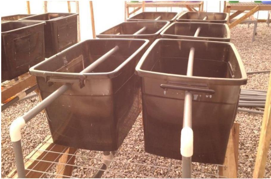
**Plate 3- 11 Setup showing inlet/feed pipes through tote box**
