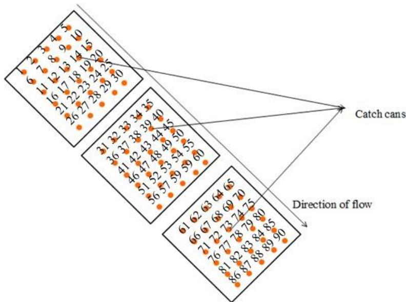
**Plate 3- 16 Grid view illustrating position of catch cans**
