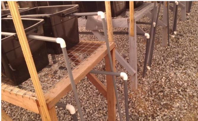
**Plate 3- 9 Setup showing feed and drain pipes**
