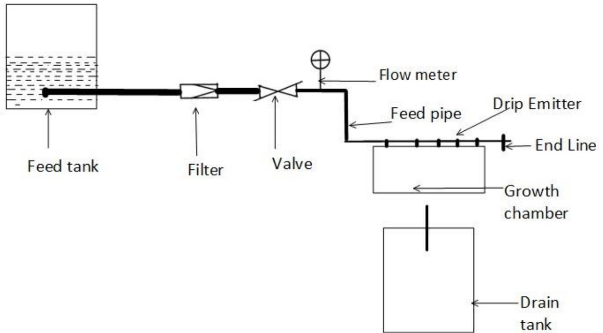
Plate 3- 5 Schematic representation of the gravity-fed system
