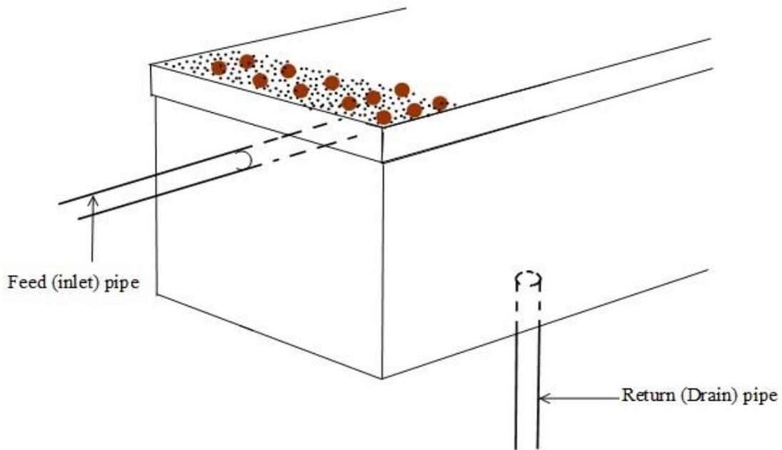
**Plate 3- 4 Feed and return pipes of the growth chamber**
