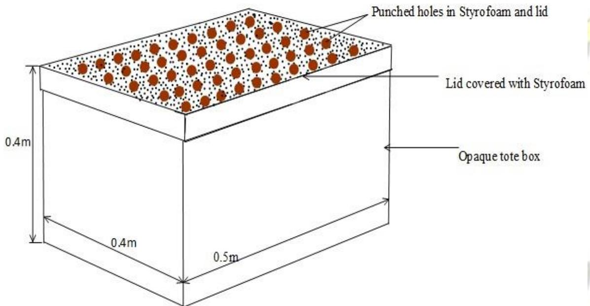
**Plate 3- 3 Design specifications of the growth chamber and plant holding tray**
