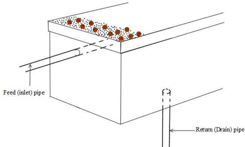
Figure 18 Feed and return pipes of the growth chamber
