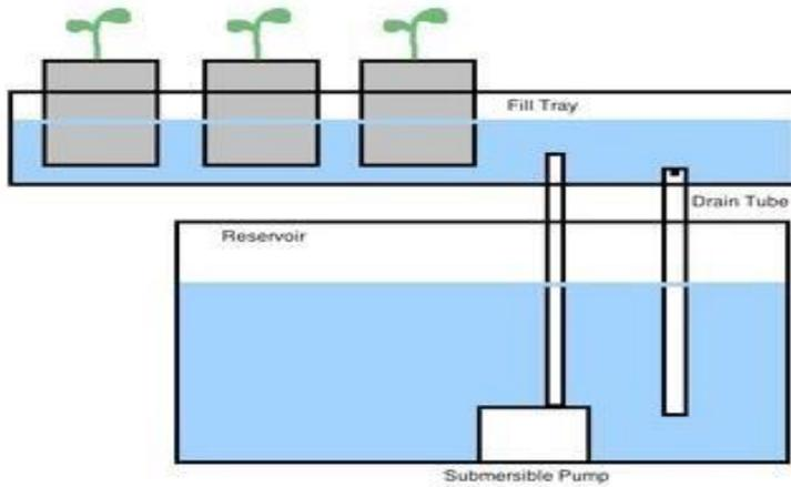
**Plate 2- 2 The ebb and flow system (Source: Hydroponics, n.d)**
