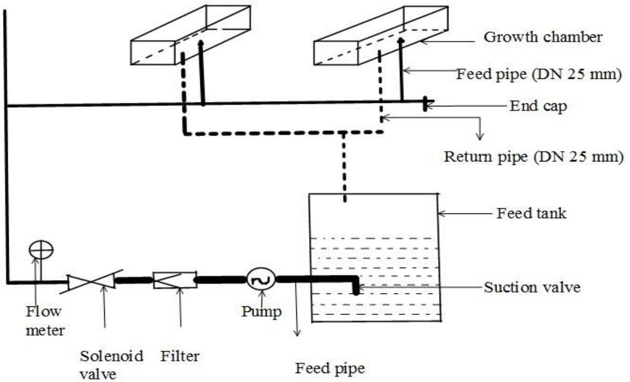
Plate 3- 1 Schematic representation of the pressurised system
