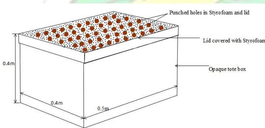
Figure 17 Design specifications of the growth chamber and plant holding tray
