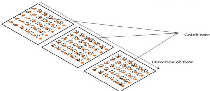
Figure 8 Grid view illustrating position of catch cans
