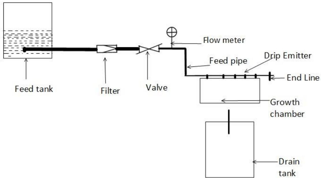
Figure 5 Schematic representation of the gravity-fed system
