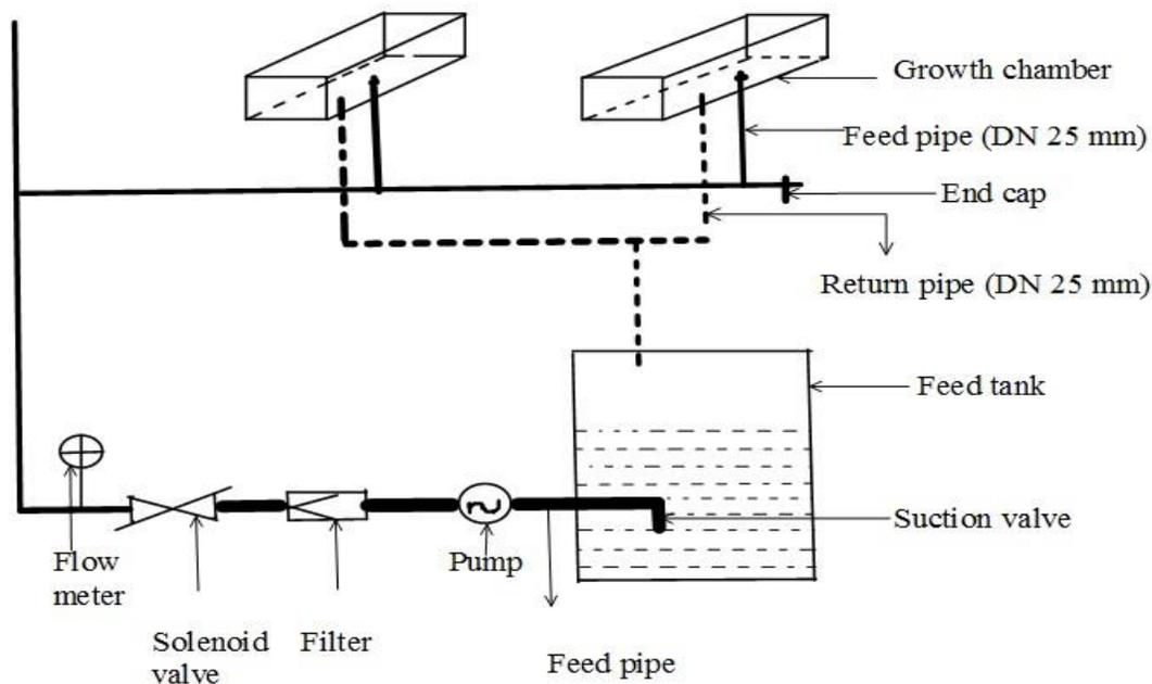
Figure 1 Schematic representation of the pressurised system
