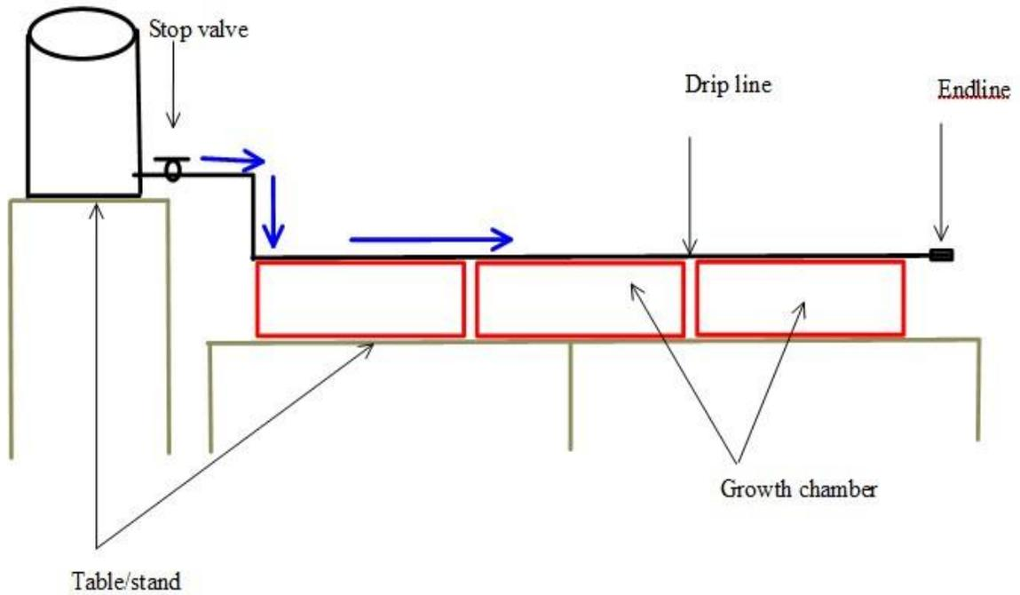
Plate 3- 6 System Flow Chart for one gravity-fed aeroponic unit
