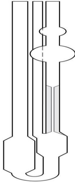
**Figure 2.4:** Schematic representation of a Ubbelohde capillary viscometer- relative viscosity of solvent in capillary (Harding, 1997)
