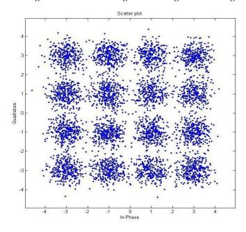
Figure 5-9 MATLAB constellation diagram showing 16-QAM constellation points
