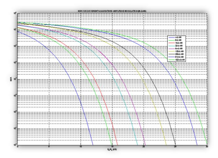
Figure 5-6 Comparison of various M-QAM modulation techniques
