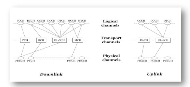
Figure 3-5 LTE Logical Transport and Physical Channel Mapping [4][23][42]
