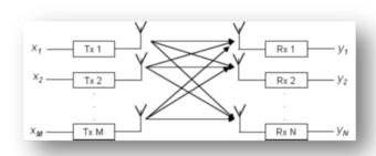
Figure 2-2 Multiple Input Multiple Outputs - MIMO
