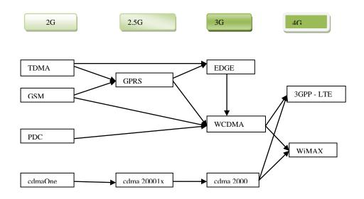
Figure 1-1 Evolution Path of Mobile Wireless Technology towards 4G
