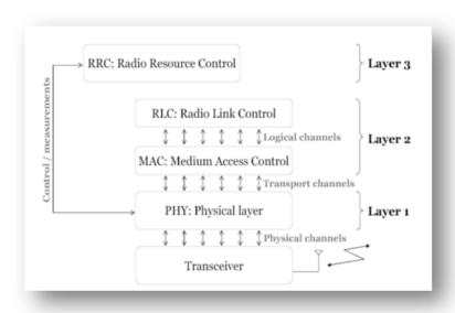
Figure 3-2 Physical layer in the UTRA protocol stack [4]
