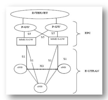
Figure 3-4 LTE simplified network architecture [2]
