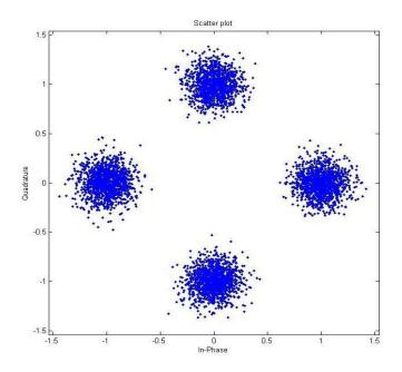
Figure 5-6 Signal Constellation Diagram showing 4-PSK using MATLAB
