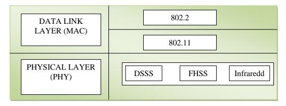
Figure 2-4 Wi-Fi physical and data link layer architecture [12]
