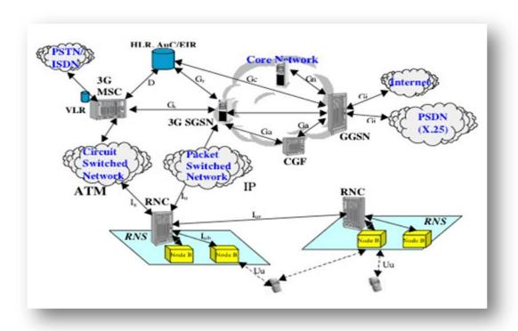
Figure 3-1 UMTS 3G Network Architecture
