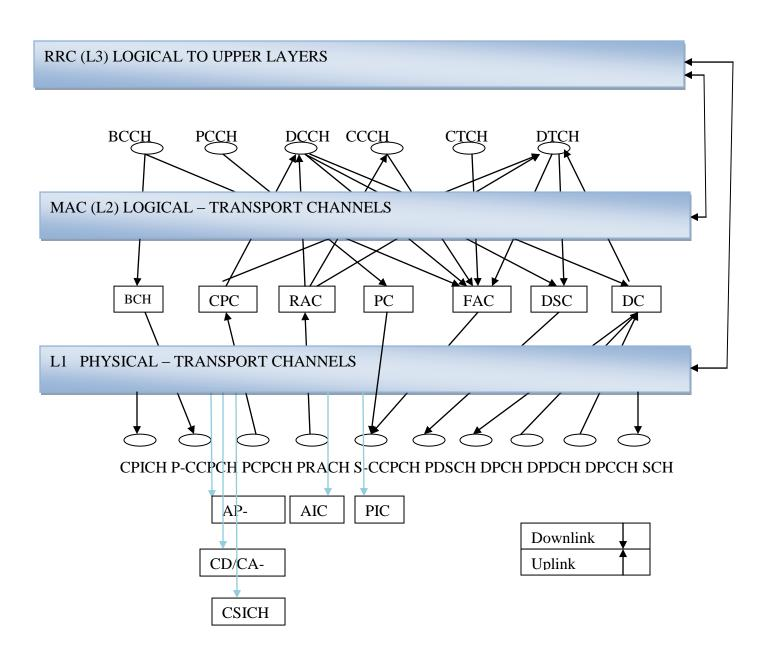
Figure 3-3 3G Logical -> Transport -> Physical Channel Mapping [32]
