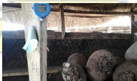
Figure 17: Data logger reading temperature and relative humidity
