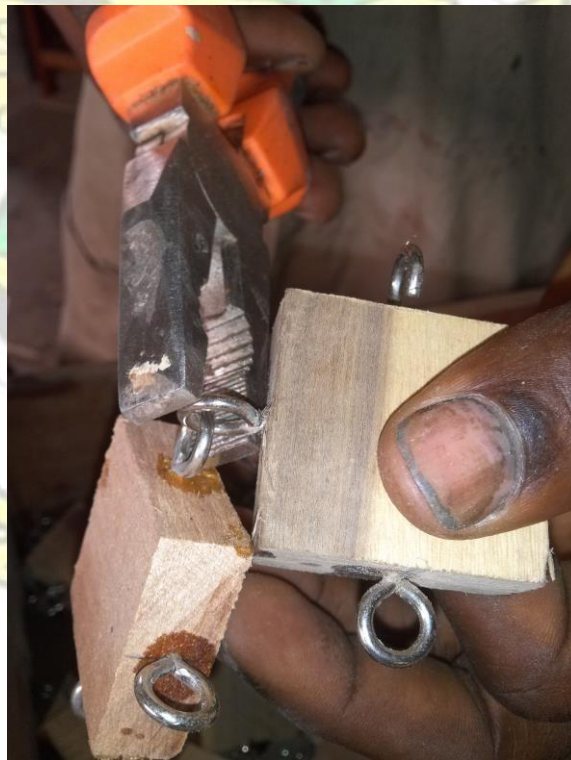
Plate 3.13: closing up the opened screw eye
