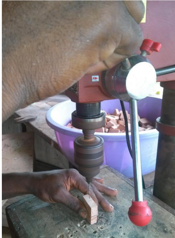
Plate 3.6 Drilling holes in the wood pieces
