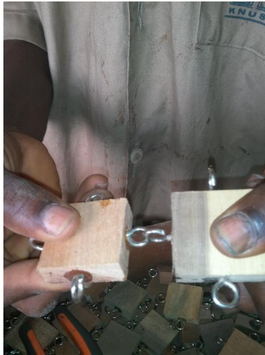
Plate 3.12: putting an open screw eye into a closed screw eye
