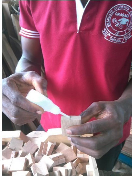
Plate 3.8 pouring super glue into the drilled holes
