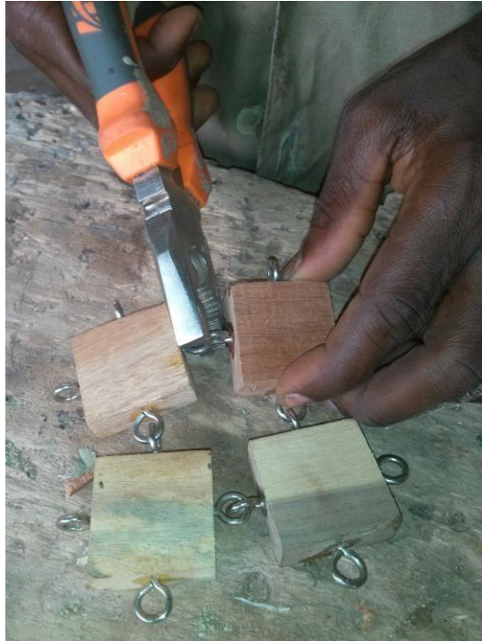
Plate 3.14: opened screw eye accepts another closed screw eye
