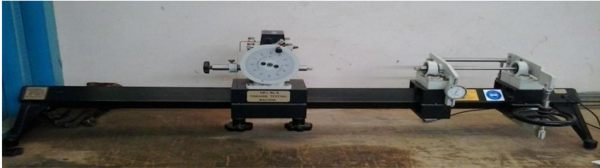
**Figure 3.5:** Tecquipment SMI MKII-torsion testing machine
