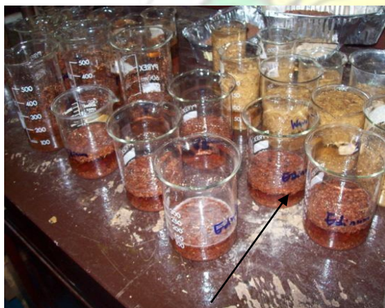
Plate 5.1 Set up for water holding capacity
