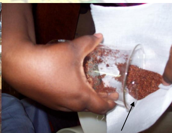
Plate 5.2 Draining of gravitational water from samples
