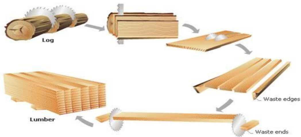
Plate 2.1 The conversion process of log to lumber showing residues produced
