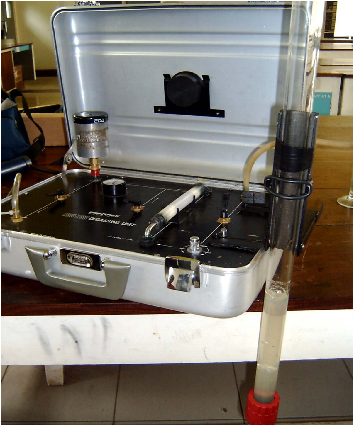
Figure 9. Radon Degassing Unit-200 with a cell and a glass tube containing sample
