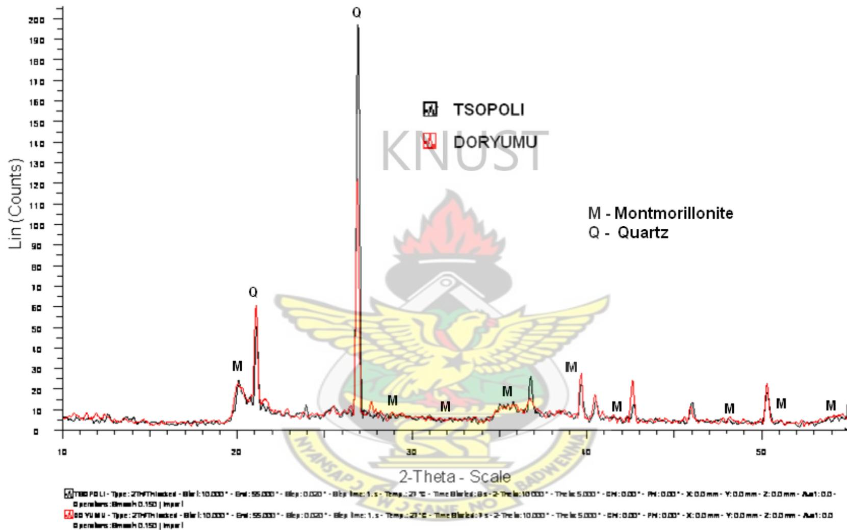
Figure 13. Diffractogram of the two soils
