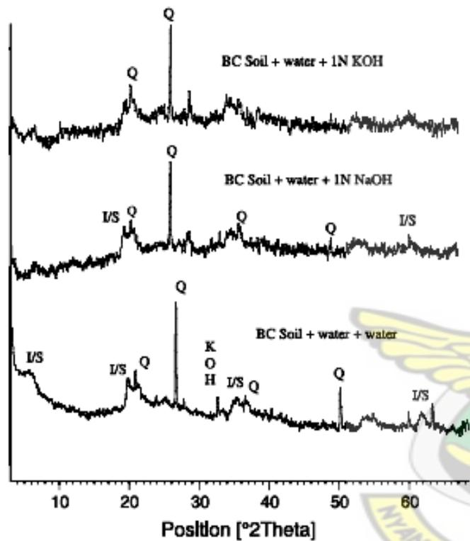
Figure 5. Typical X-ray diffractogram of black cotton soils (from Sivapullaiah and Reddy, 2010)
