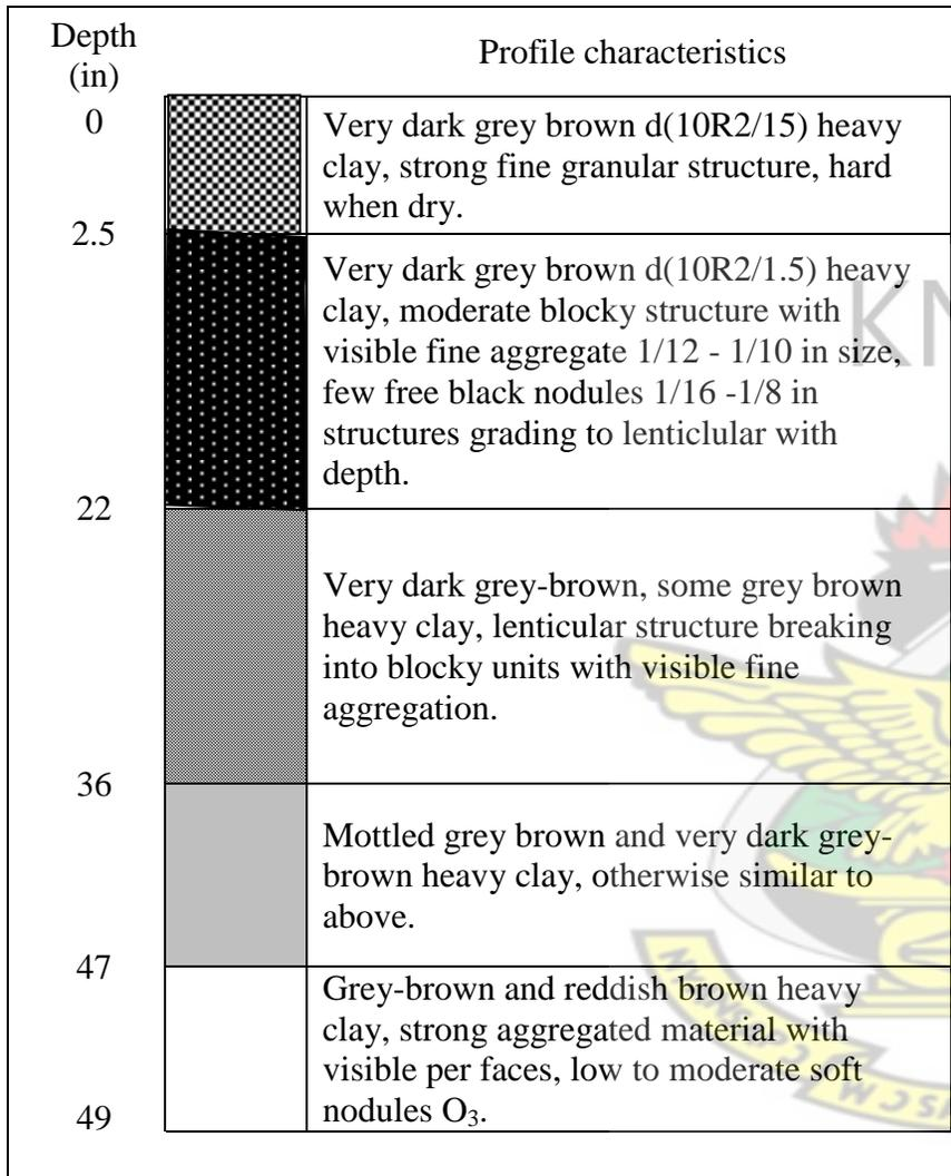
Figure 4a. Typical black cotton soil profile from Australia (Aitchison, et al., 1962)
