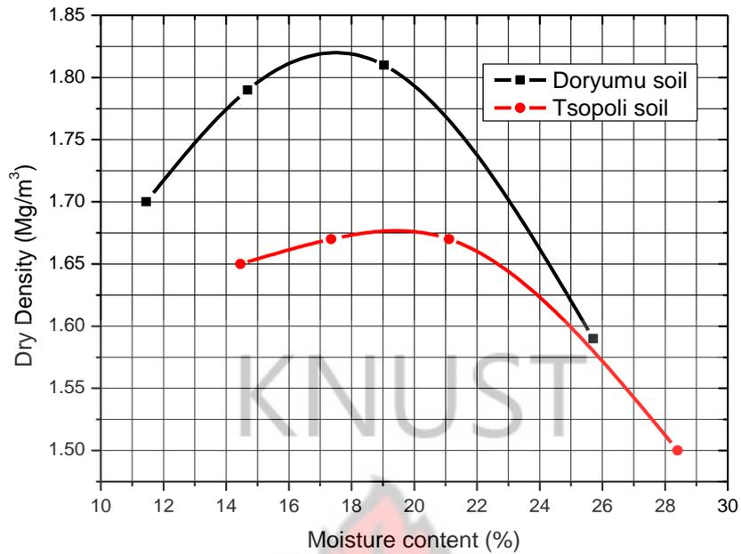
**Figure 17. Compaction characteristics of the black cotton soils**
