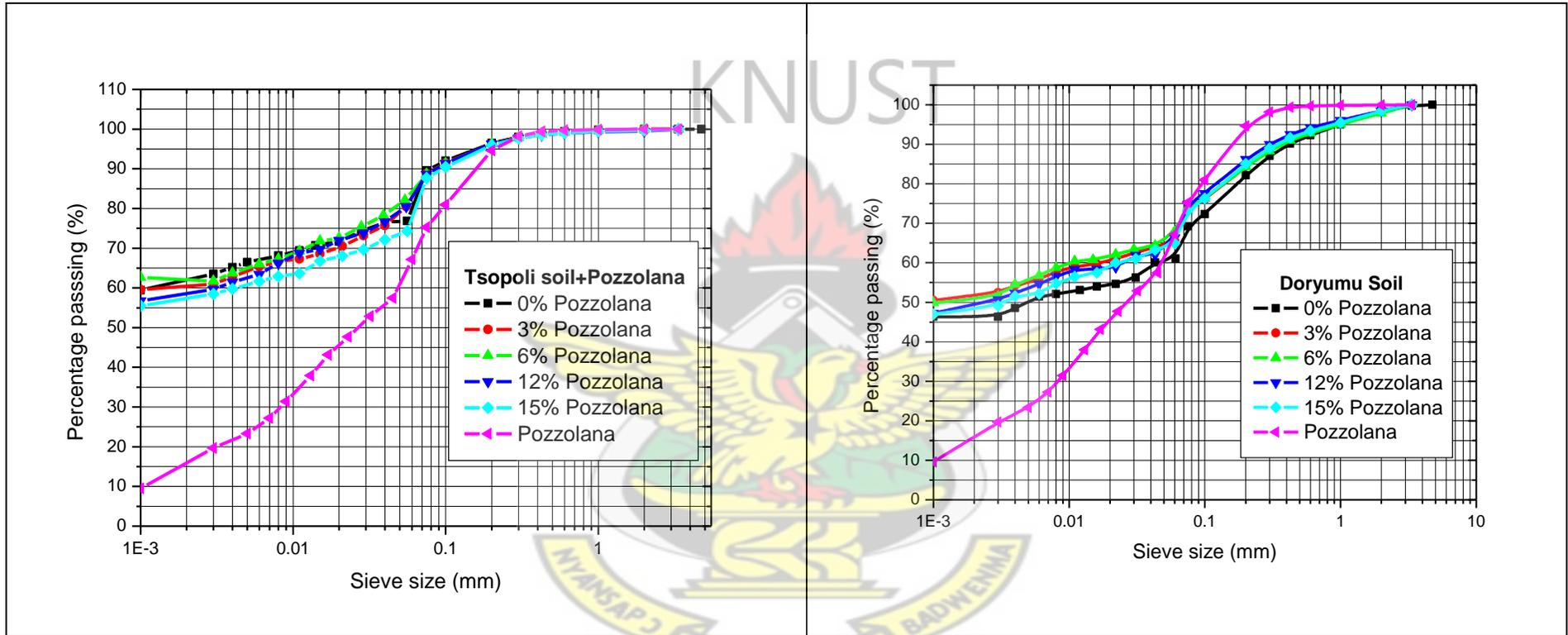
Figure 26. The particle size distribution curves of the pozzolana stabilised soils
