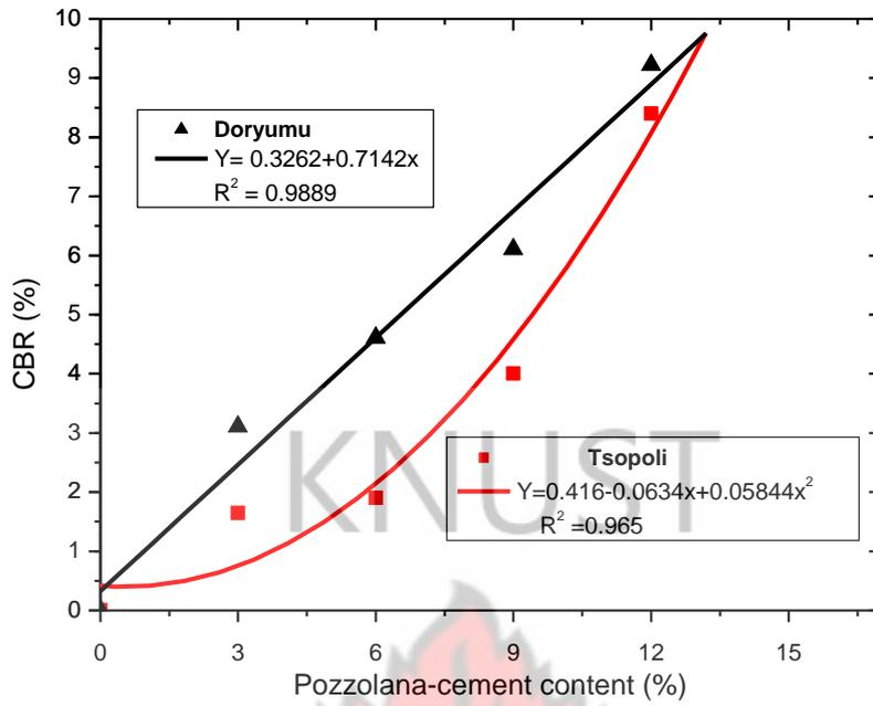
Figure 40. Variation of CBR value with Pozzolana-cement content of the soils
