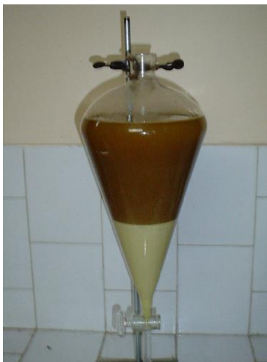
Fig. 3.2: Washing of Biodiesel.
