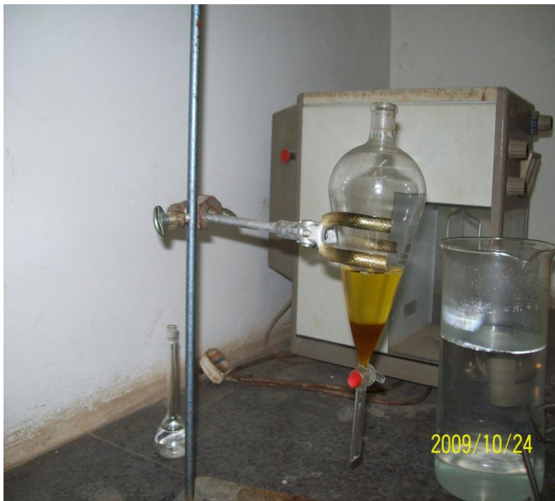
Fig. 3.1: Setup showing crude ester layer on top and glycerol layer at the bottom.
