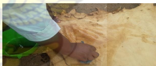
Application of oil for fatliquoring
