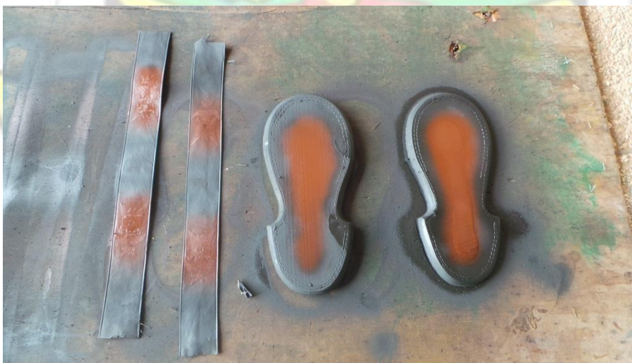
Plate 30: Showing a brown paint sprayed on the uppers and the soles.
