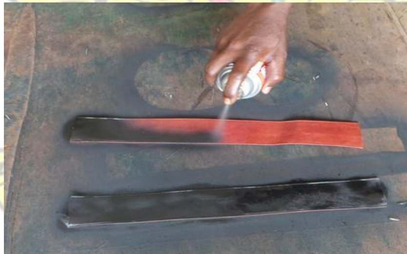
Plate 32: Showing uppers being sprayed with black
