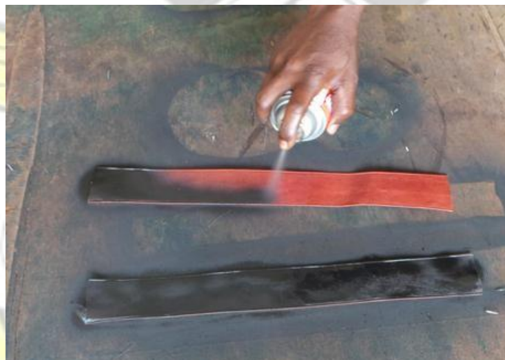
Plate 40: Showing the uppers being sprayed with black colour
