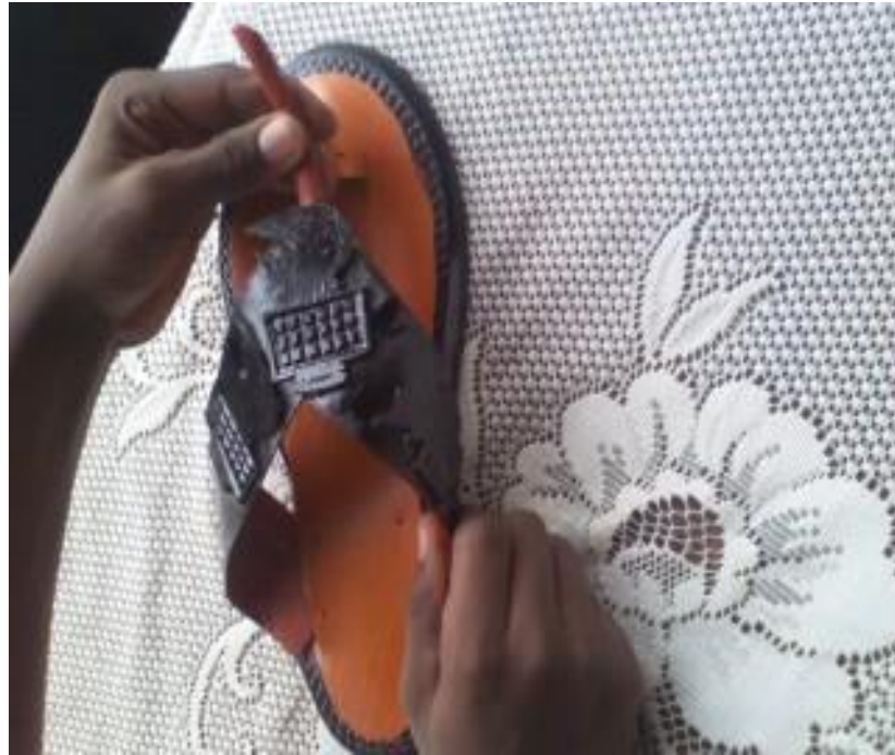
Plate 23: Showing the uppers being fixed onto the sole.
