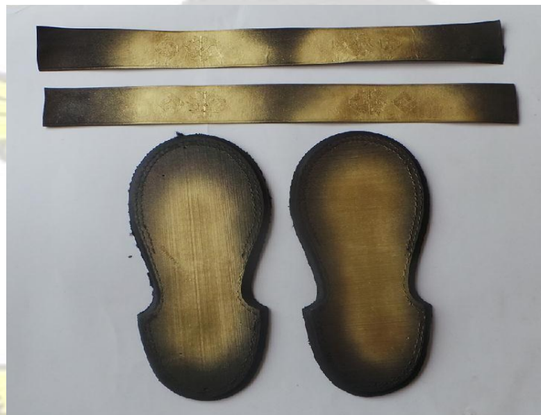
Plate 34: Showing a yellow paint sprayed on the uppers and the soles
