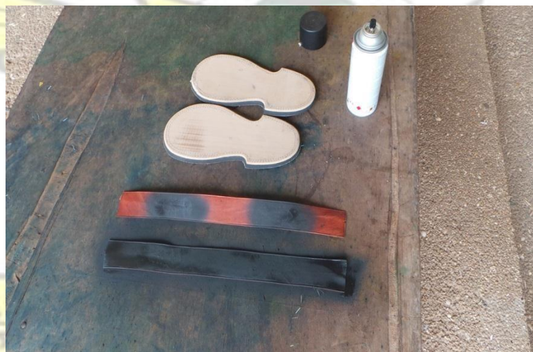
Plate 44: Showing the uppers with cut out masking tape and sprayed
