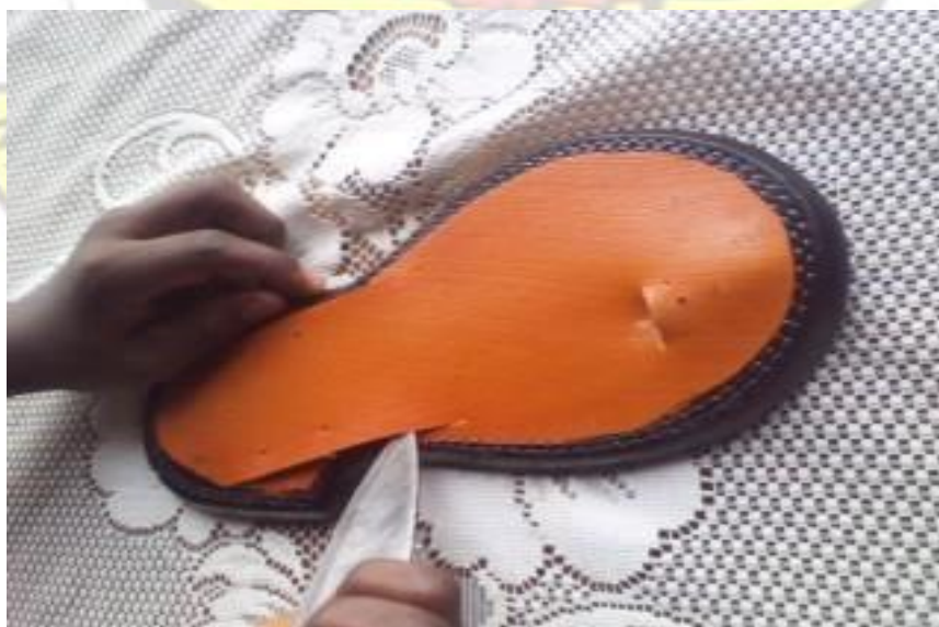
Plate 22: Incising where to fix the uppers on the buna
