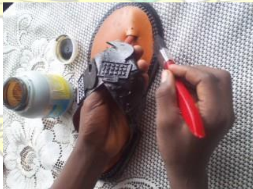
Plate 24: Showing application of jet on an _ahenema' footwear
