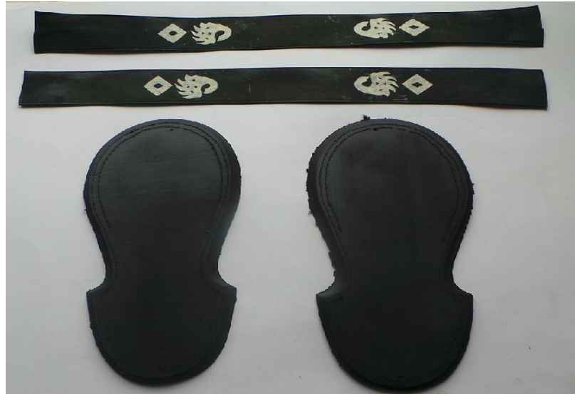
Plate 33: Showing the motif cut out from the masking tape on the uppers
