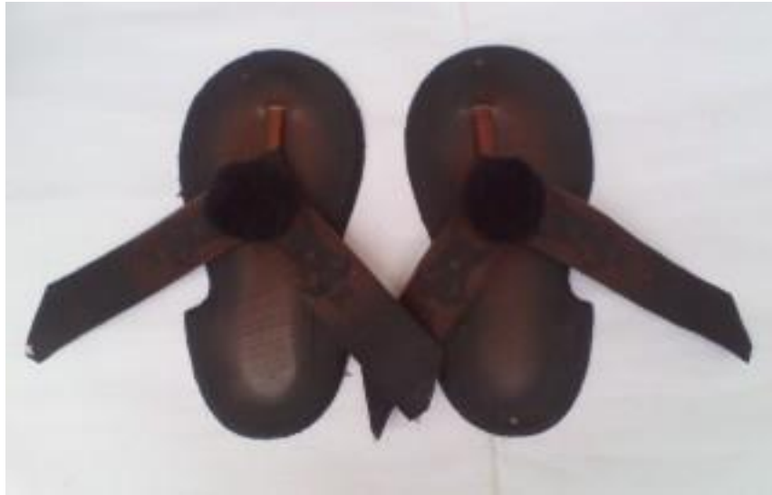
Plate 31: Uppers ready to be fixed onto the sole
