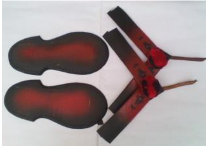
Plate 39: Showing the uppers ready to be fixed onto the sole
