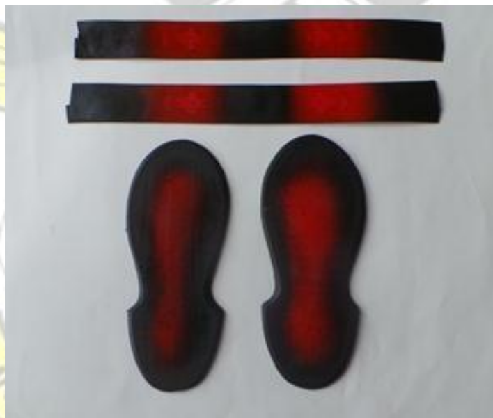
Plate 38: Showing the uppers and the soles sprayed with red colour
