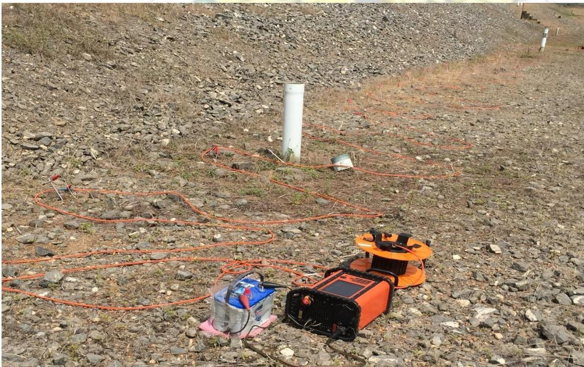
Plate 4.1 Measurement of resistivity and induced polarization in progress
