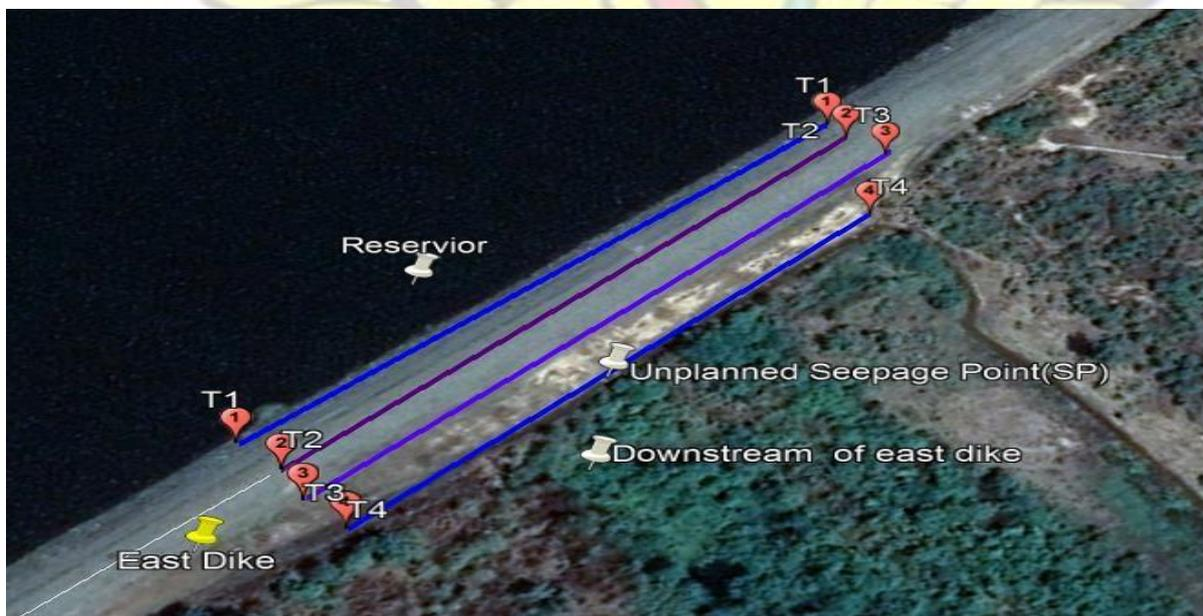
Figure 4.1 Orientation of traverse lines
