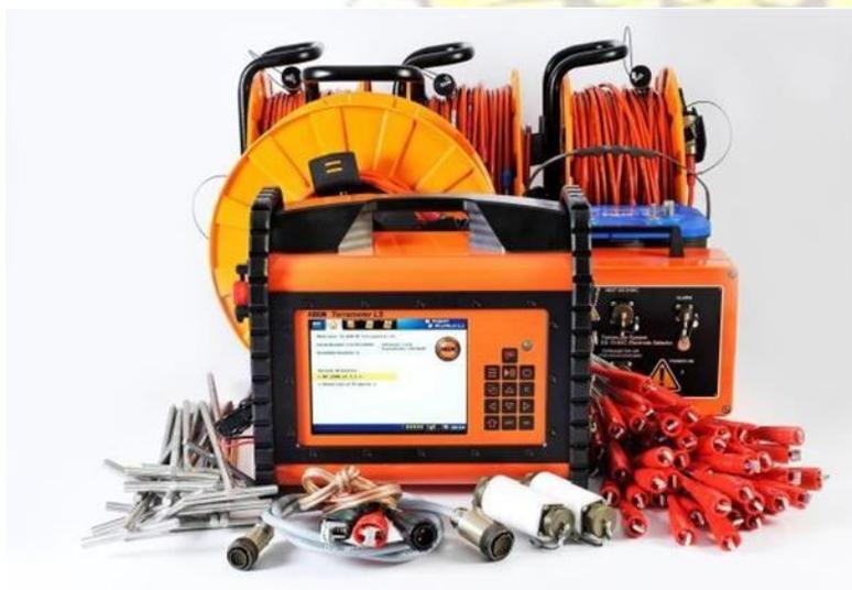
**Figure 2.10 Geoelectrical imaging system with Terrameter LS**
