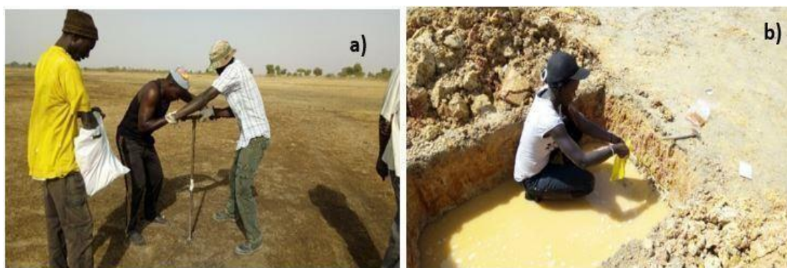
Figure 3.1: Soil sampling by auguring (a) and sample pits (b)
