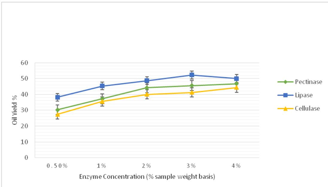
Figure 4.4: Effect of enzyme concentration on oil recovery.
