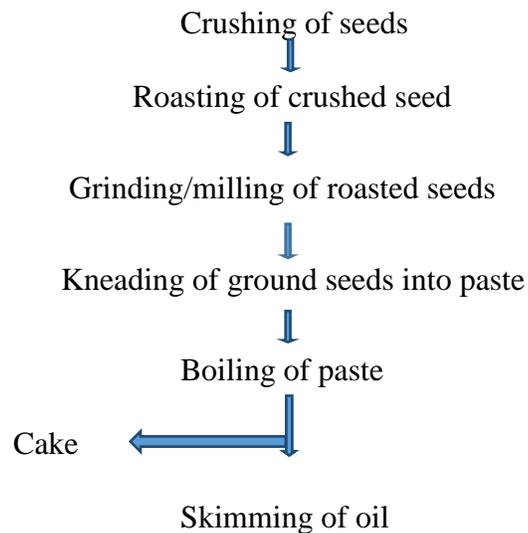
Figure 2.4 Simplified flow chart of the HWF method of oil extraction
