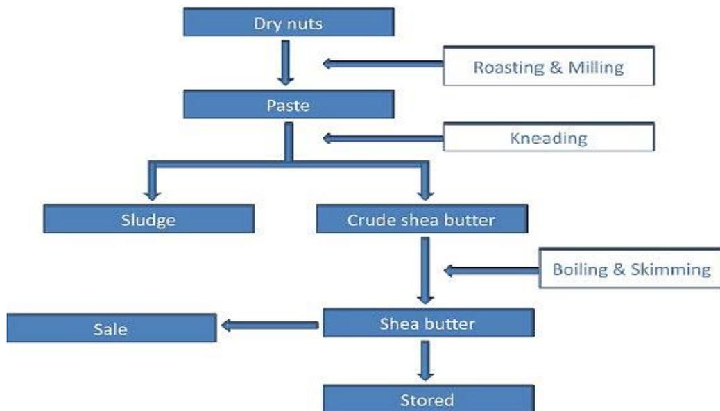
Figure 2.3: Flow Chart for Local Processing of Shea Butter
