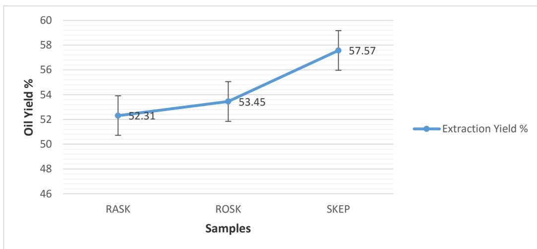
**Figure 4.2:** Oil recovered using solvent (n-hexane) extraction method.
