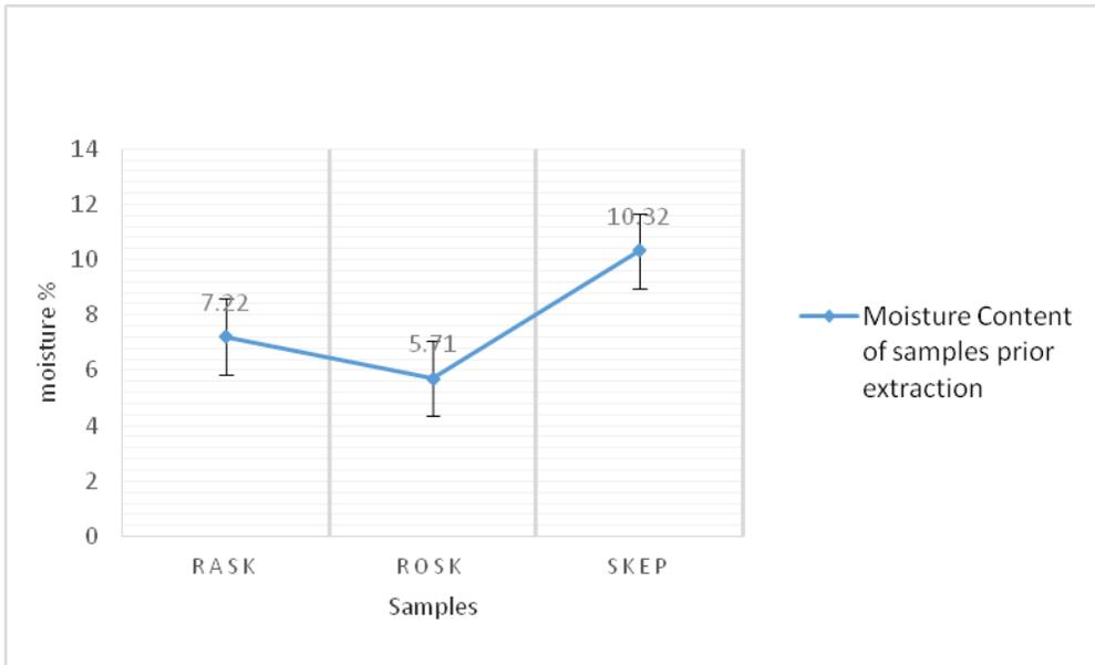
**Figure 4.1:** Percentage Moisture Content of Pre-treated Shea Samples Prior to Shea butter Extraction
