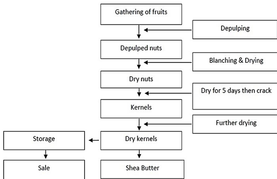
Figure 2.2. Flow Chart for Local Collection and Pre-treatment of Shea Nuts
