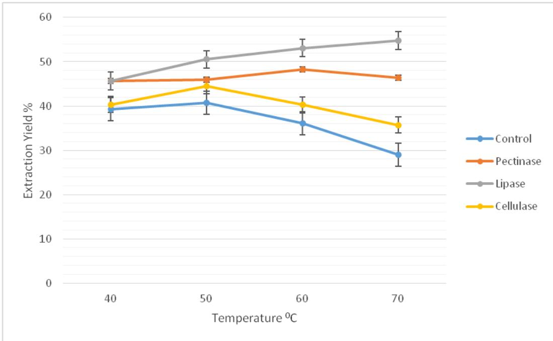
Figure 4.6: Effect of temperature on extraction yield
