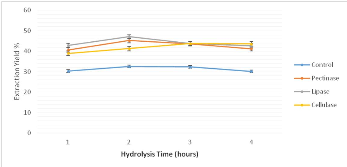
**Figure 4.3: Effect of Hydrolysis time on Shea Butter Extraction Yield**
