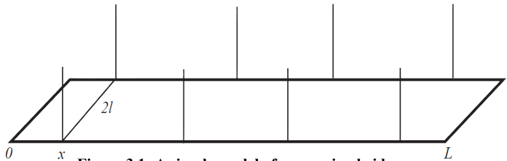
Figure 3.1: A simple model of suspension bridge
