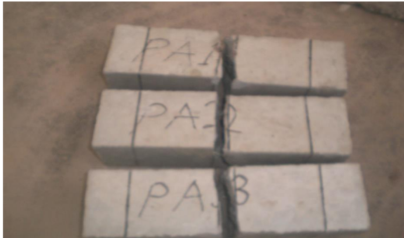
Figure 4.3: Plain concrete prisms after failure
