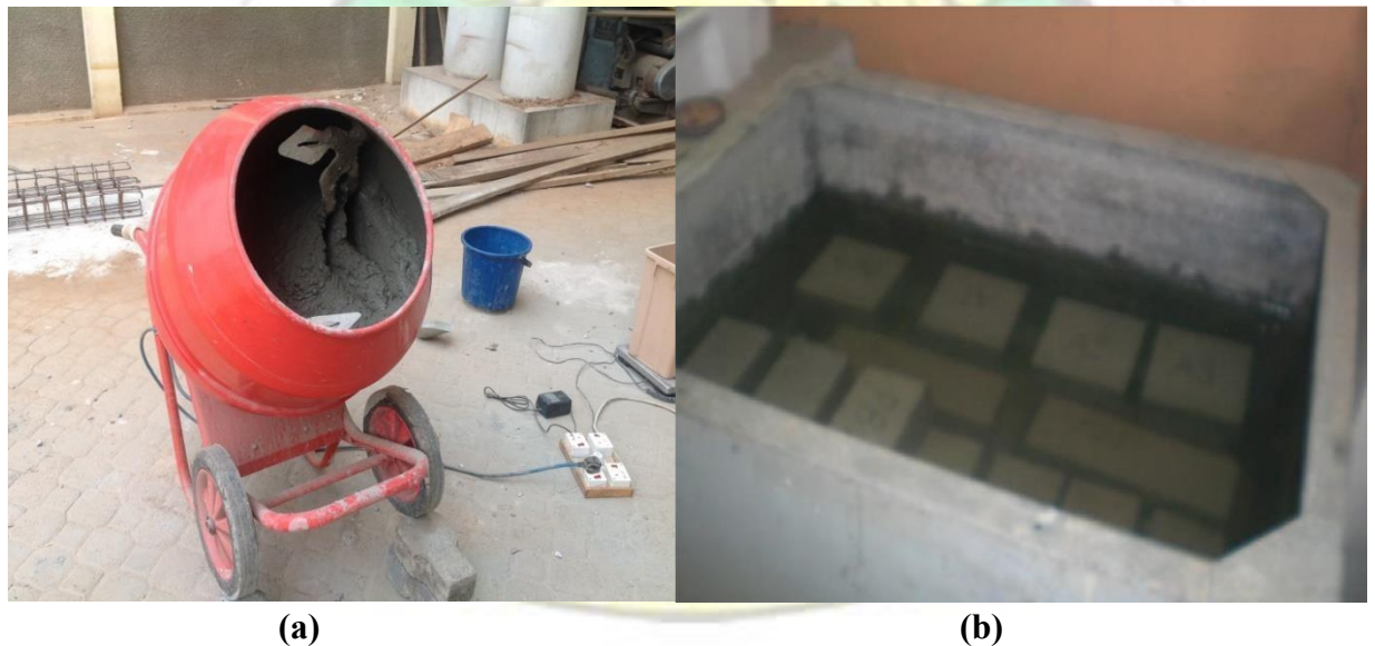
Figure 3.2: a) Portable electric concrete mixer in operation during concrete mixing and b) Curing of test cubes and prisms in a steel curing tank.
