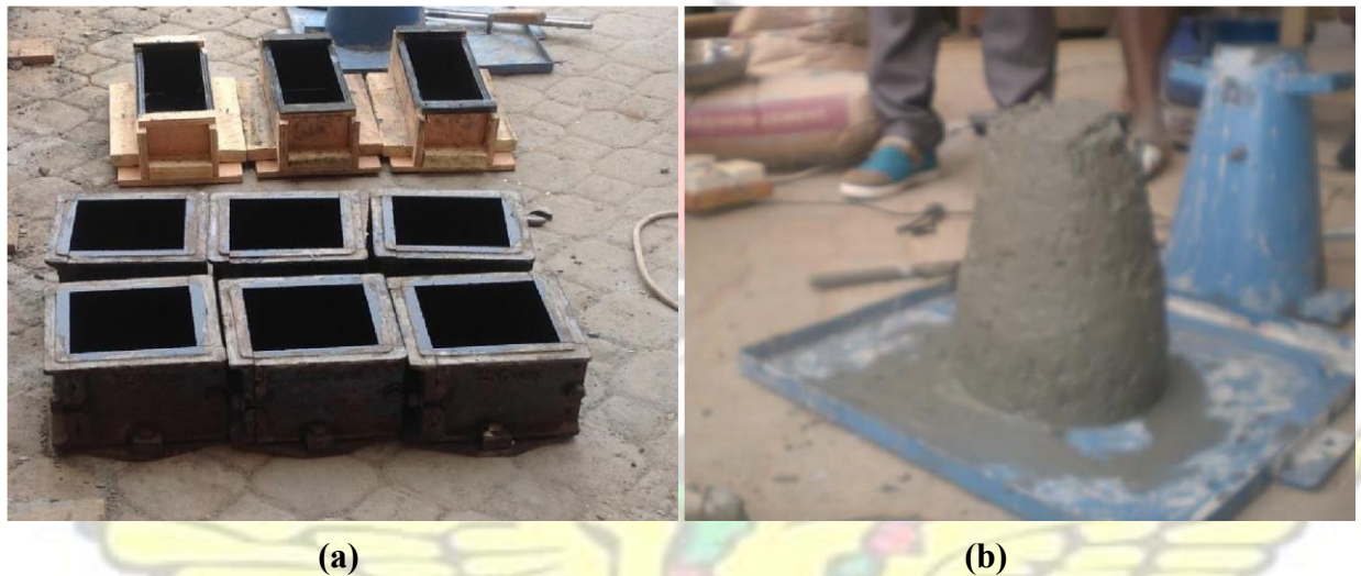
Figure 3.1: a) Steel and wooden moulds/ formwork for casting concrete cubes and prisms and b) Slump test for checking consistency and workability of concrete.
