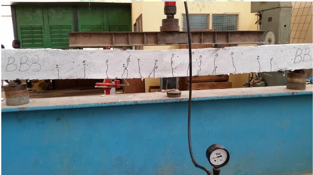
Figure 4.12: Crack propagation and characteristics of the control specimen
