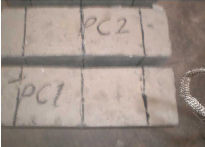
Figure 4.5: 0.50 percent fibre concrete prisms after failure
