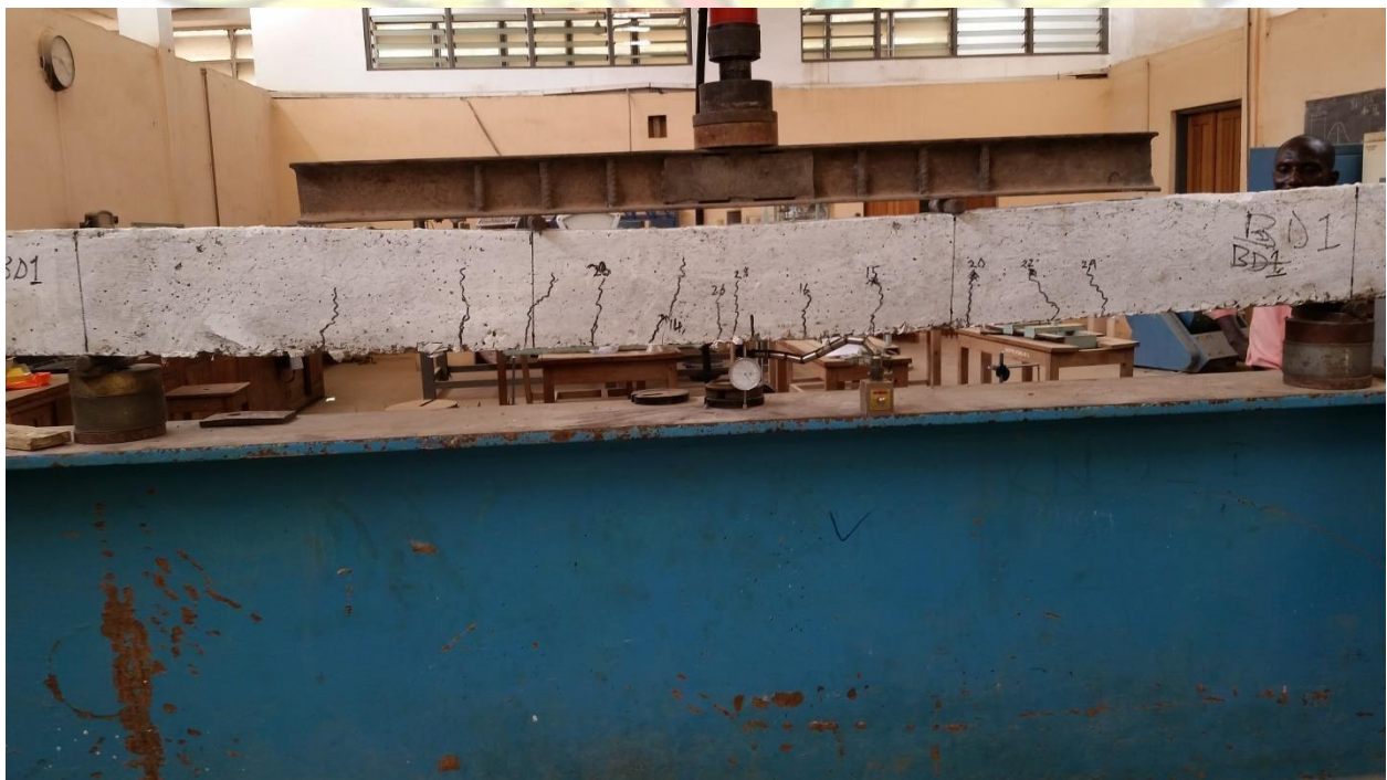
Figure 4.15: Crack propagation and characteristics of the 1.0% fibre concrete
