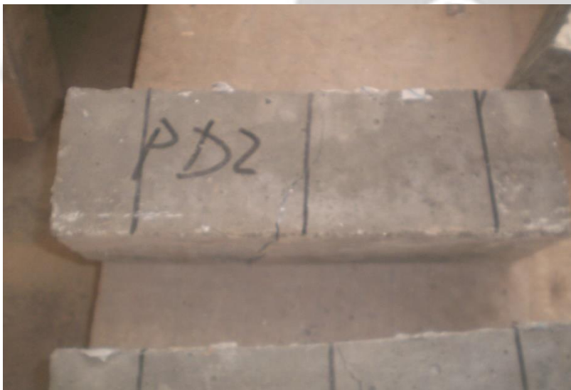
Figure 4.6: 1.0 percent fibre concrete prisms after failure
