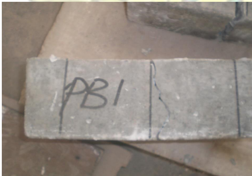
Figure 4.4: 0.25 percent fibre concrete prisms after failure
