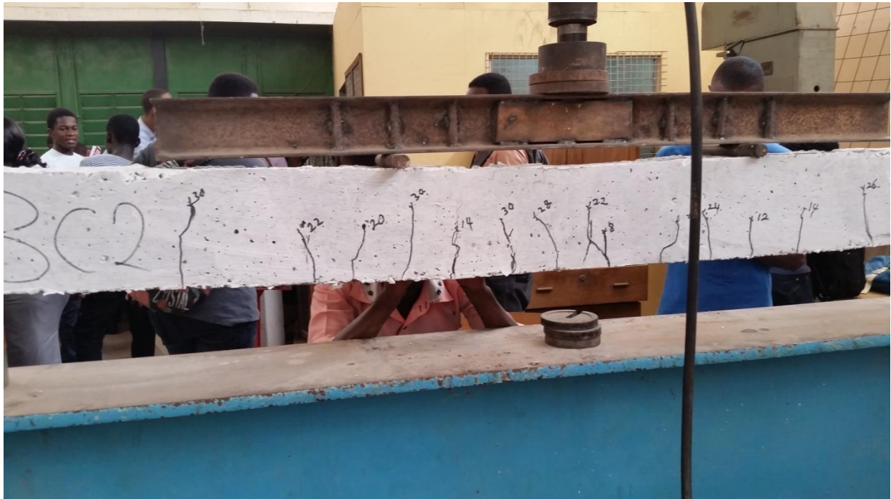
Figure 4.14: Crack propagation and characteristics of the 0.5% fibre concrete
