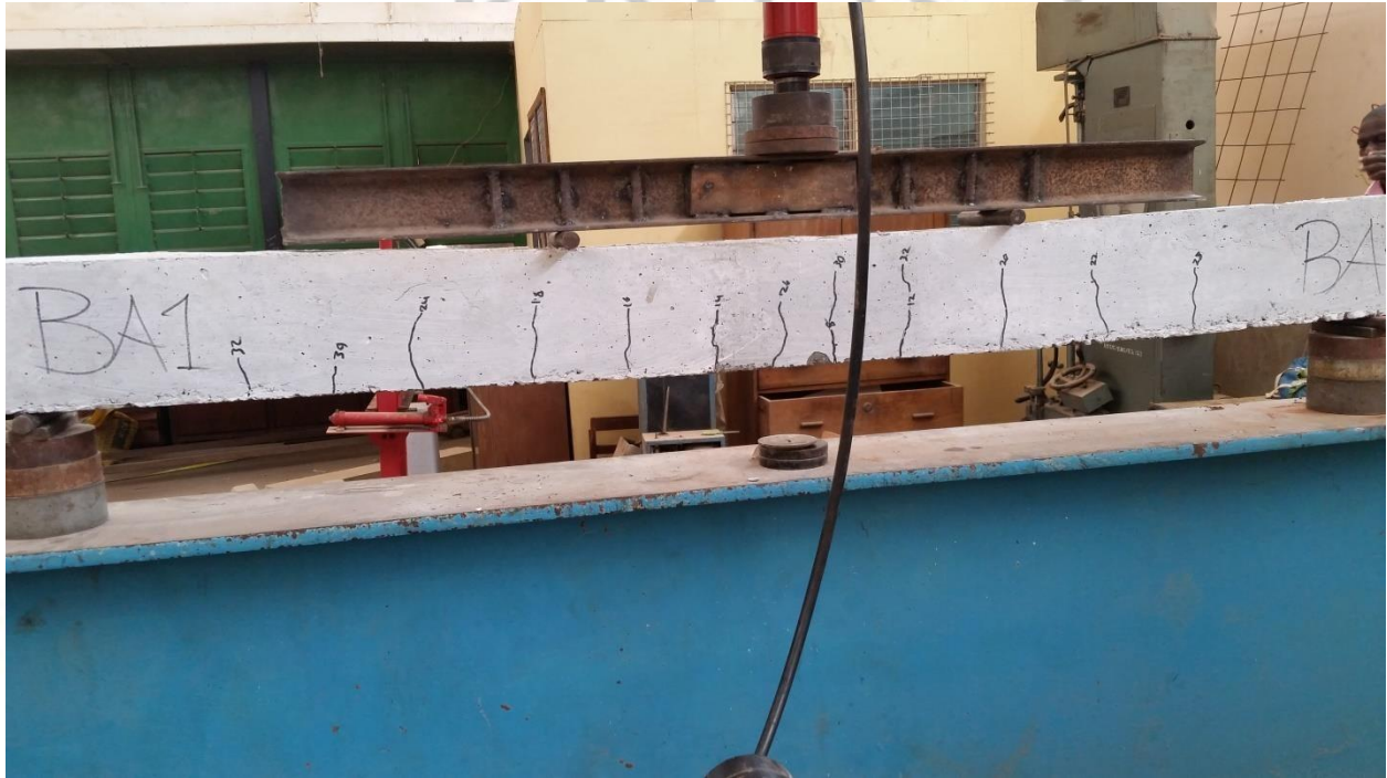
Figure 4.12: Crack propagation and characteristics of the control specimen
