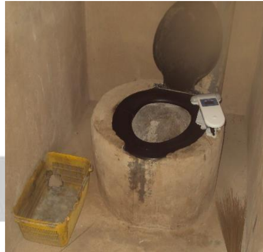
Figure 3-5: Positioning of gas detector to take measurements in a VIP latrine
