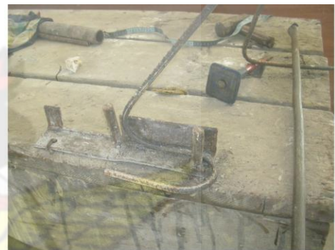
Plate lviii: Researcher using the bending bar to bend the metal in the bending stake
