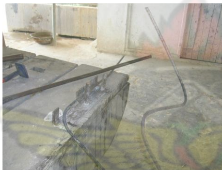
Plate lviii: Researcher using the bending bar to bend the metal in the bending stake
