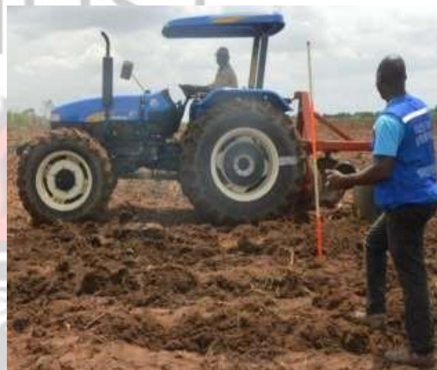
Measurement of wheel-slip with ridger in tillage position
