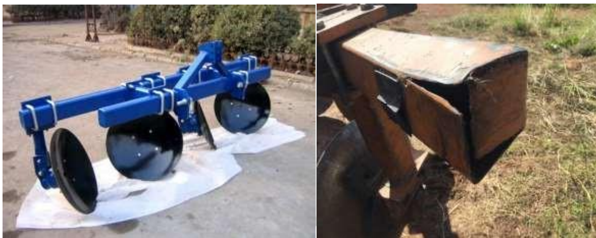
Plate 2.2: a. Two-row disc ridger made in China, b. Defects associated with disc ridger
