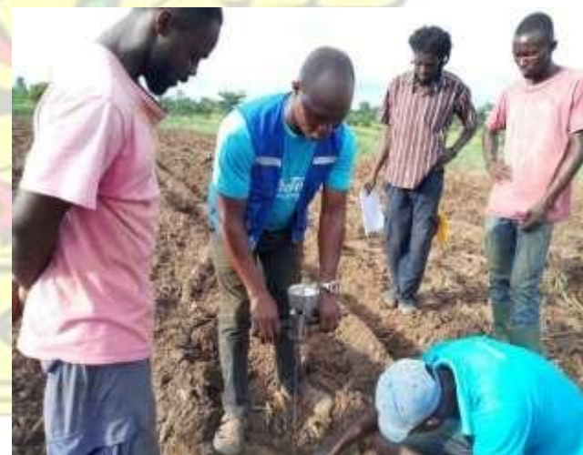
Measurement of soil penetration resistance after ridging
