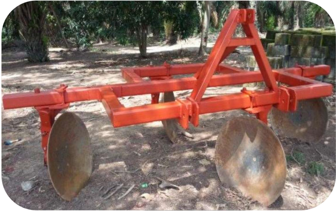
Plate 4.1: The fabricated fully-mounted double row disc ridger ready for testing
