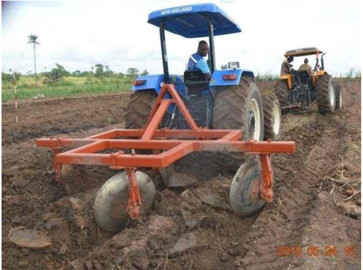
Plate 3.3: Tractors–dynamometer, implement mounted in tillage operation.
