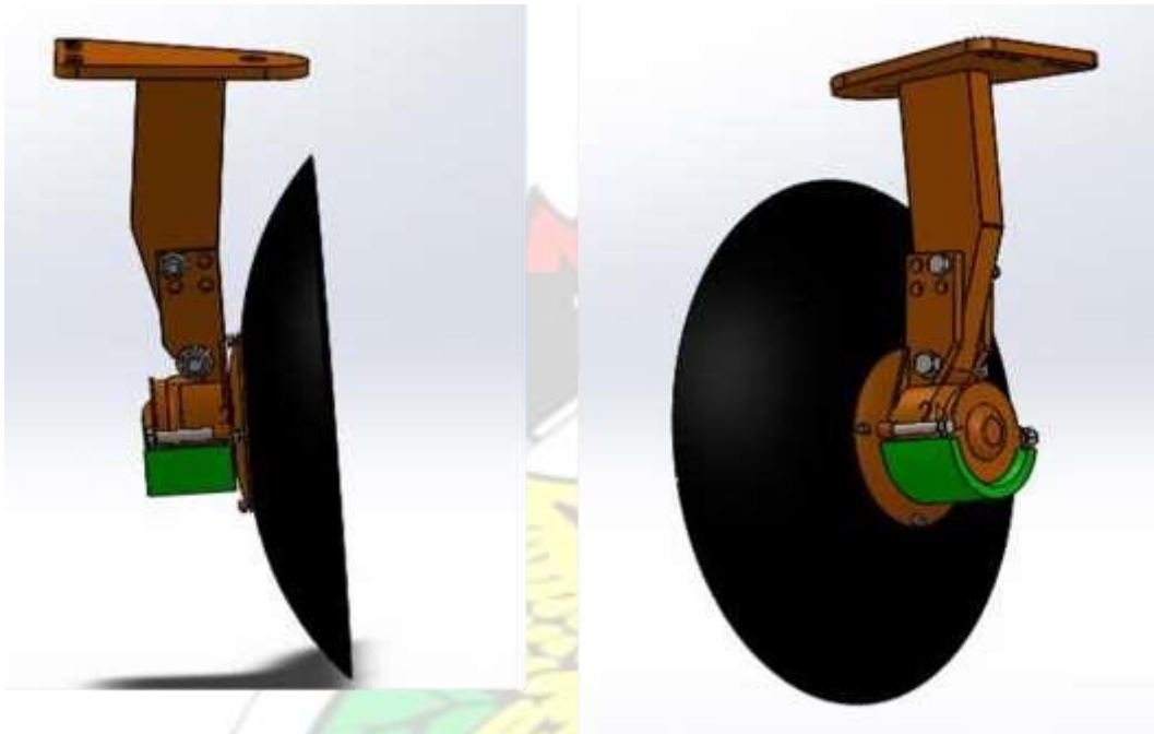
Figure 3.10: 3D views of the ridger bottom sub-assembly
