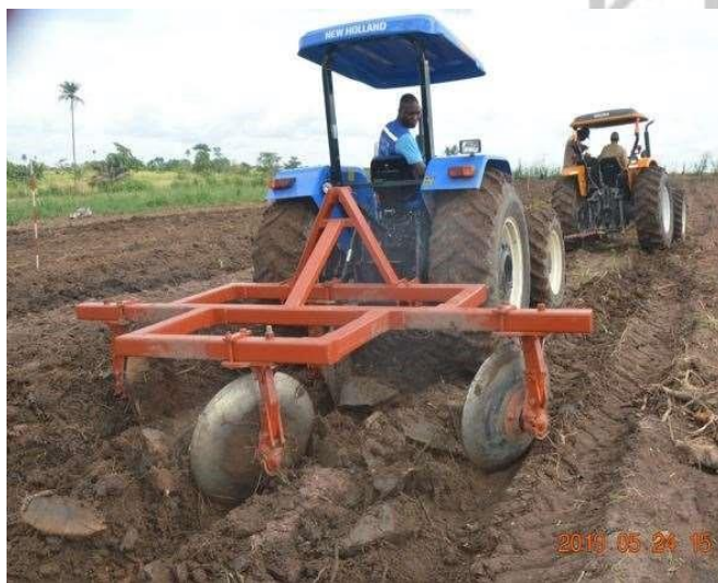
Measurement of draught with ridger in tillage position
