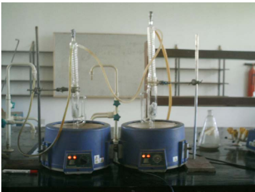
Plate IV. Soxhlet apparatus in use (for extraction)
