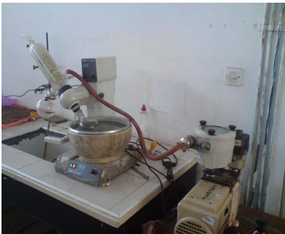
Plate V. Rotary evaporator in use (to concentrate extract)
