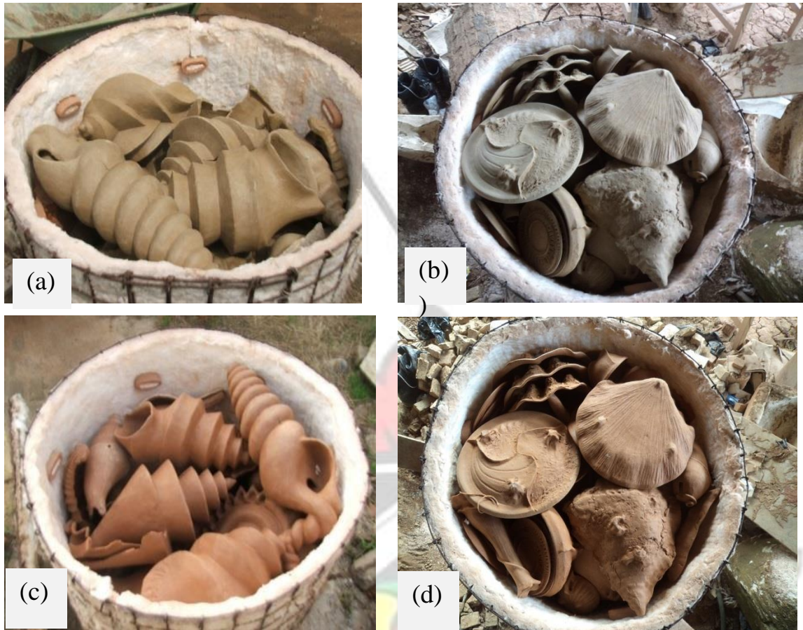
Plate 3- 16: The ceramic seashells (a) and (b) Shells in bone dry state and (c) and ( d) Shells in bisque state using the gas kiln
