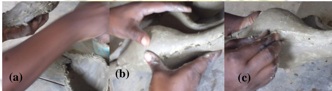
Plate 3- 8: Cleaning of fettles (a) Applying clay slip to the seams of the shells (b) Joining two halves to get a full shell (c) Removing fettles at the ridges.
