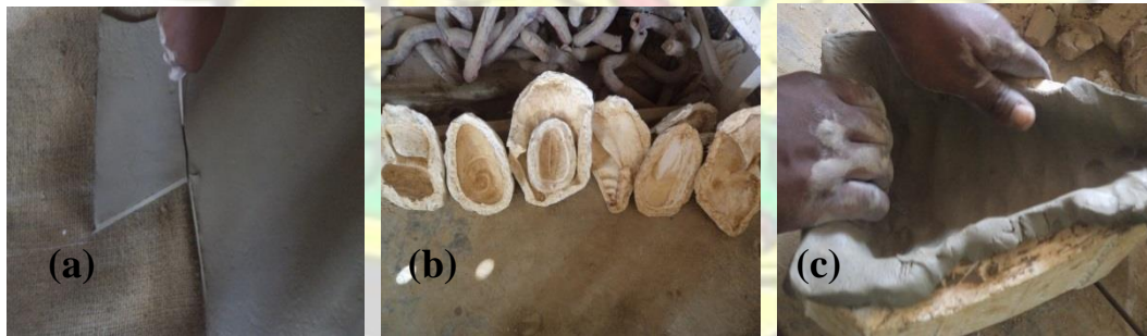
Plate 3- 6: (a) Clay slab (b) P.O.P moulds (c) Pressing clay slab into the mould
