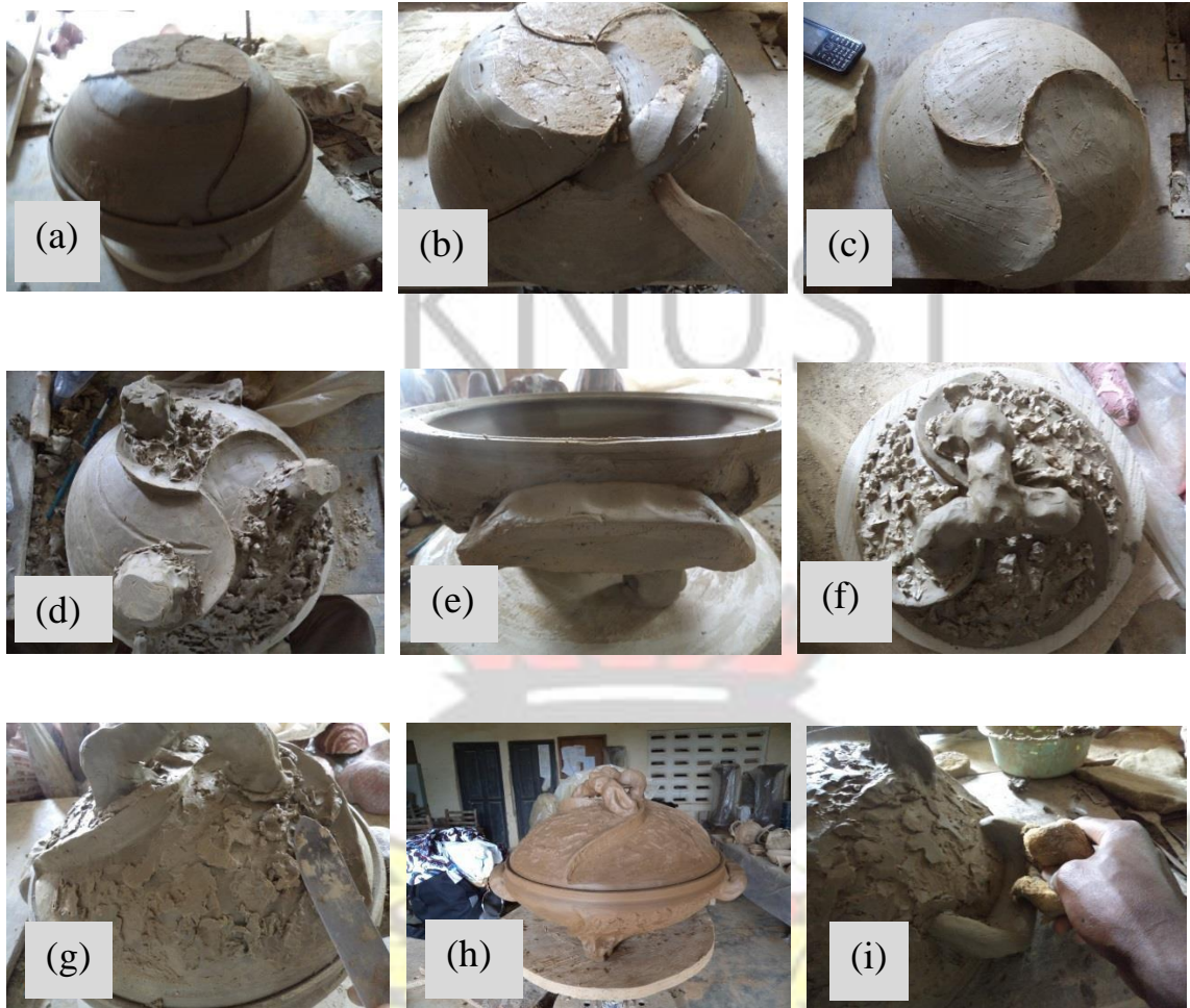
Plate 3- 14: Pictures showing the making of the serving bowls (a) thrown bowl and lid (b) demarcated lines for the foot and handle (c) demarcated lines for foot and handle (d) fixing of foot (e) fixed handles on the bowl (f) fixed handle on the lid (g) decorating with a knife (h) finished bowl with lid (i) cleaning with a foam.
