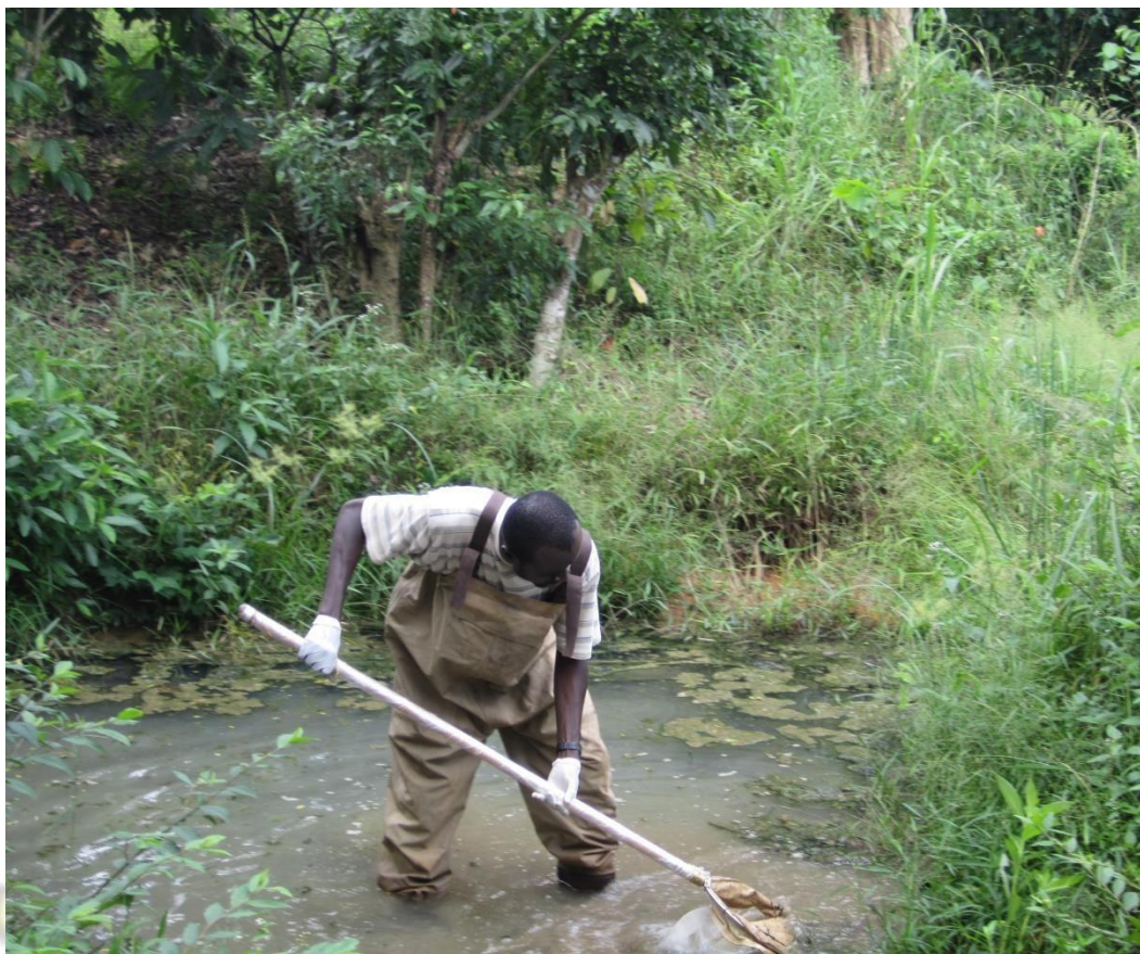
Figure 3.5 Collection of invertebrate samples using the D-frame net (Author, 2012).
