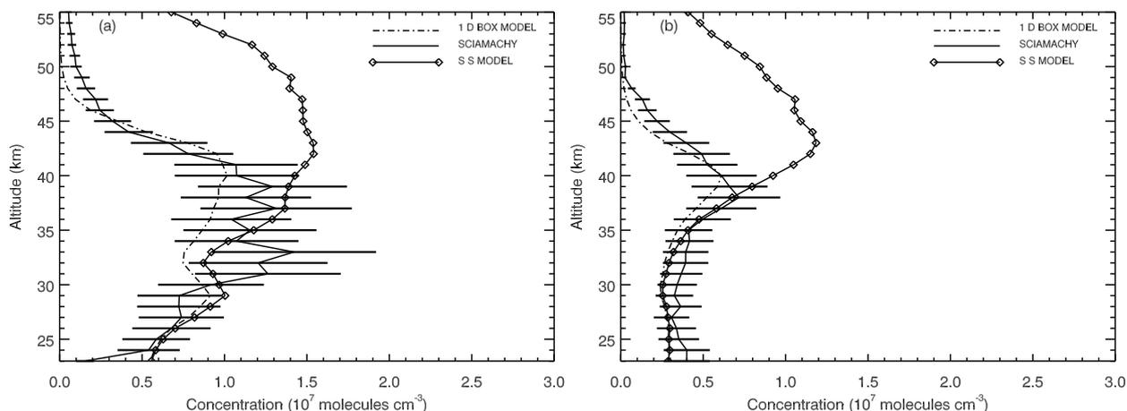
Figure 14. NO<sub>3</sub> profile retrieved compared with NO<sub>3</sub> profile calculated from the photochemical and steady state models. Solid line is the retrieval result, the dashed-dotted line is the photochemical model output and the solid line with diamond points is the steady state model results. (a) Example of NO<sub>3</sub> profiles for 14th March, 2003 (at SZA of 110°). (b) Example of NO<sub>3</sub> profile for 12th April, 2003 (at SZA of 115°).
