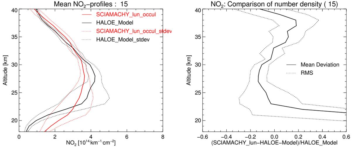
Figure 12. Left: mean  $\text{NO}_2$  profile and corresponding standard deviation for 15 co-located events in 2003, SCIAMACHY version 2.2 in red and HALOE in black. Right: the mean relative deviation (solid line) and the standard deviation of the relative deviation (dotted line).
