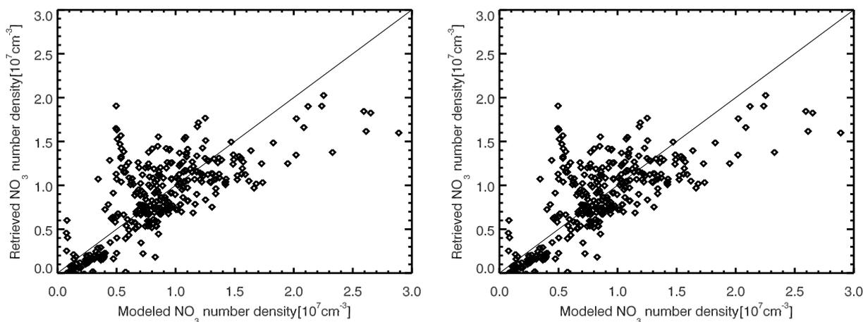
Figure 15. Retrieved NO<sub>3</sub> concentration from SCIAMACHY lunar occultation as a function of NO<sub>3</sub> calculated from the steady state model output. (a) The result for latitude band of (60–65° S), the correlation coefficient for this graph is 0.83. (b) The result for latitude band of (66–72° S) the correlation coefficient for this graph is 0.98
