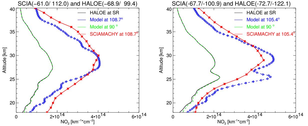
Figure 11. Examples of  $\text{NO}_2$  profiles from SCIAMACHY lunar occultation version 2.2 compared with HALOE for 2003 (left) and 2004 (right). Red the SCIAMACHY result, blue the HALOE photochemically scaled to SCIAMACHY SZA, green the model result at HALOE SZA, and black the HALOE  $\text{NO}_2$  profile.
