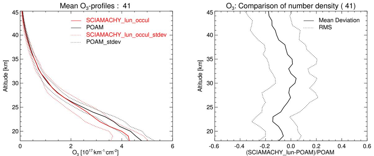
Figure 10. *Left:* SCIAMACHY-POAM mean ozone profiles for 2003 (41 coincidences). *Right:* the mean relative deviations (solid line) and the standard deviations of the relative deviations (dotted line) of the 41 SCIA-POAM III co-located observations.
