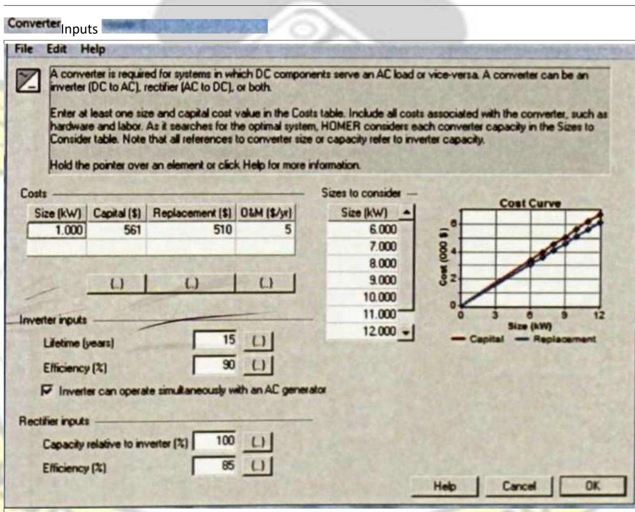
Figure 5.4 : sample of converter input
