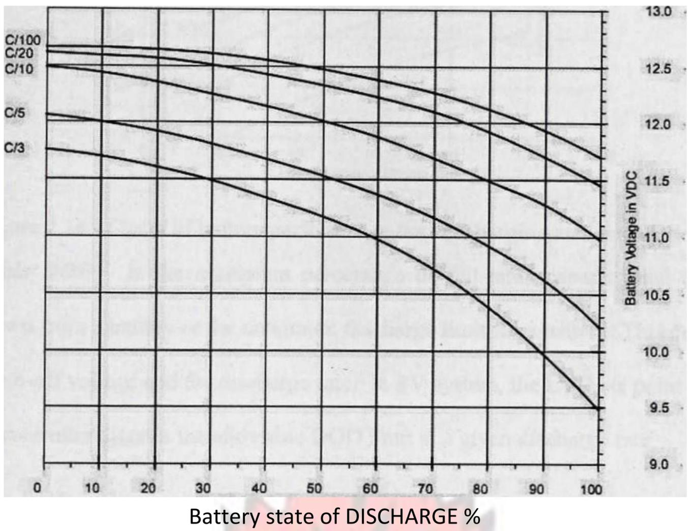
Figure 2713 - Graph of Voltage versus energy delivered from the battery
