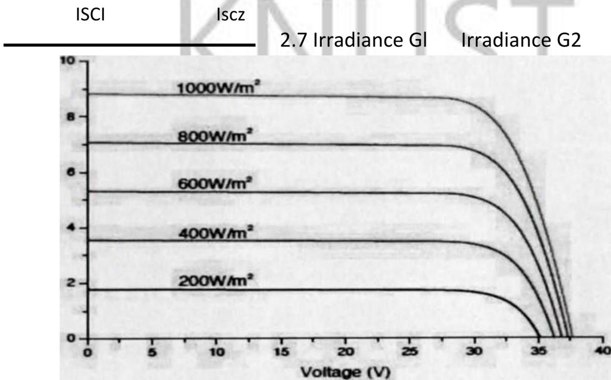
Figure 2.10 - Effect of irradiance on current and voltage Source: ( Savana Solar, 2013)
