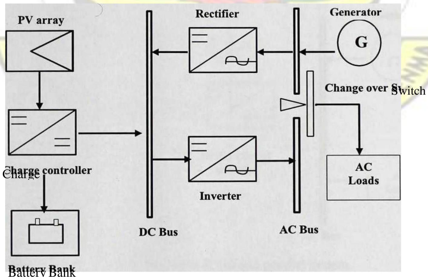
Figure 2.3 schematic of hybrid solar PV/diesel switched system
