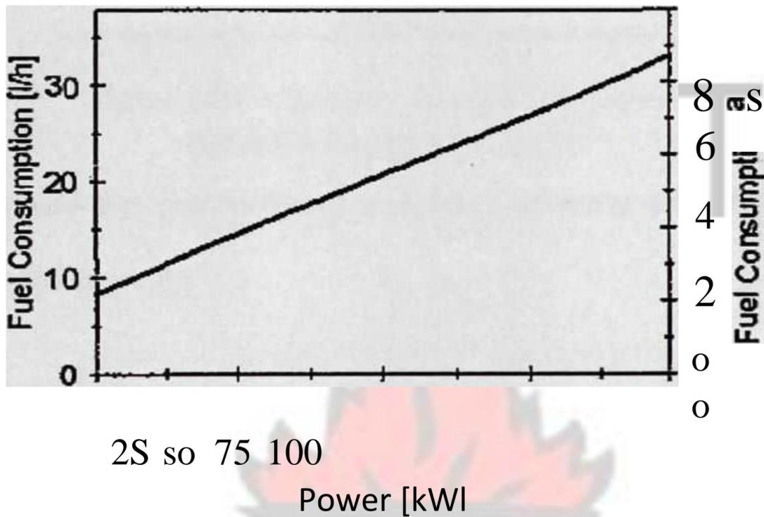
Figure 2.17 - Diesel fuel consumption and electrical power output curve (Barley, et al., 1995)
