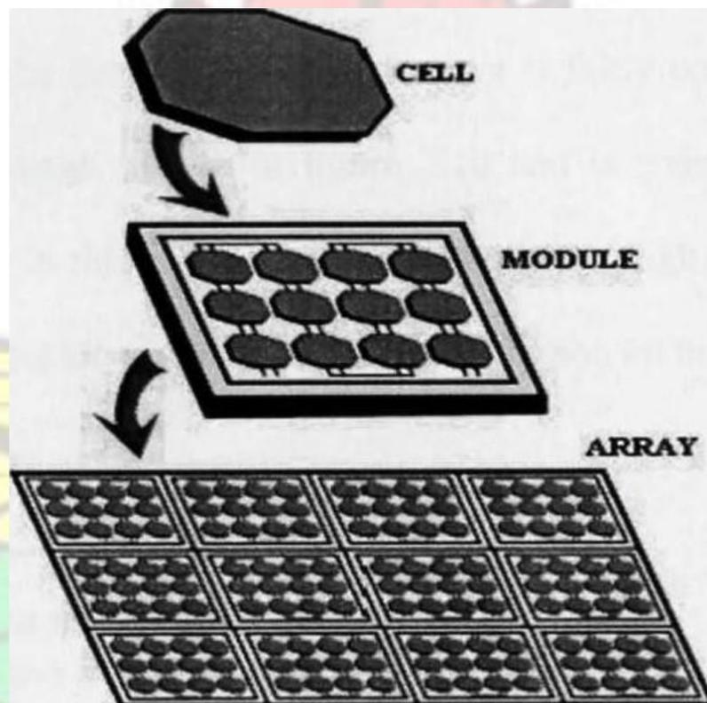
Figure 2.8- Solar cell, Module and Array
