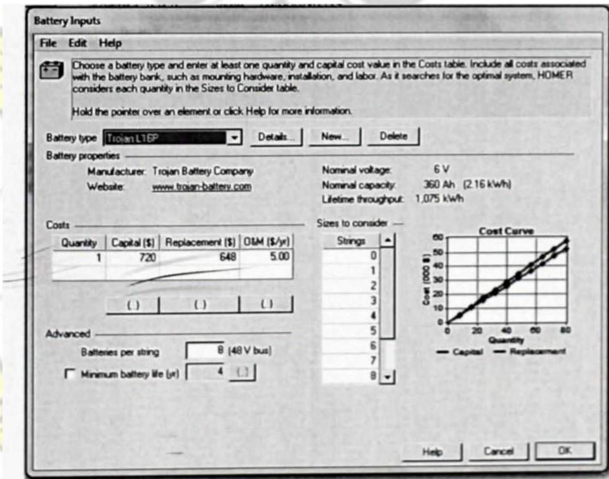
Figure 5.6 Sample of battery input
