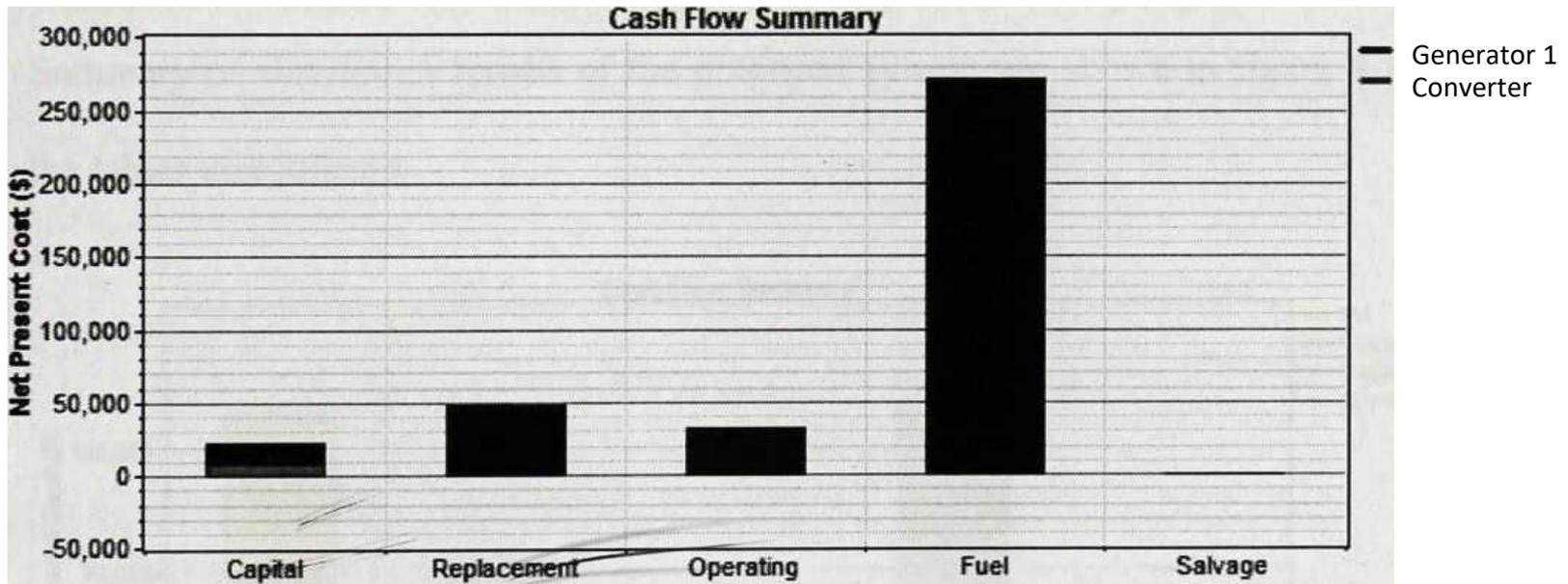
Figure 4.3 - Bar chart showing Cash flow summary of diesel only system.
