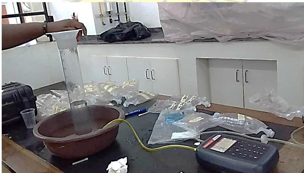
Plate 3.2: Liquid displacement method
