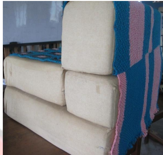
Plates 3.40 and 3.41 Different Parts of the Covering being Pinned onto Sofa
