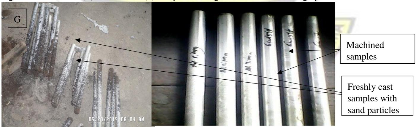
Figure 3-5 Picture of (G) samples fresh out of mould and (H) machined samples with good finish
