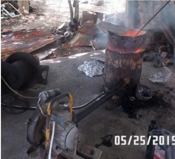
Figure 3-1 Fuel fired lift out crucible furnace used for the melting operation
