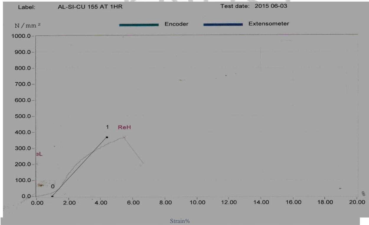
Figure 4-36 Stress-strain graphs for Al-Si-Cu alloy at 155 °C artificially aged for 1 hour
