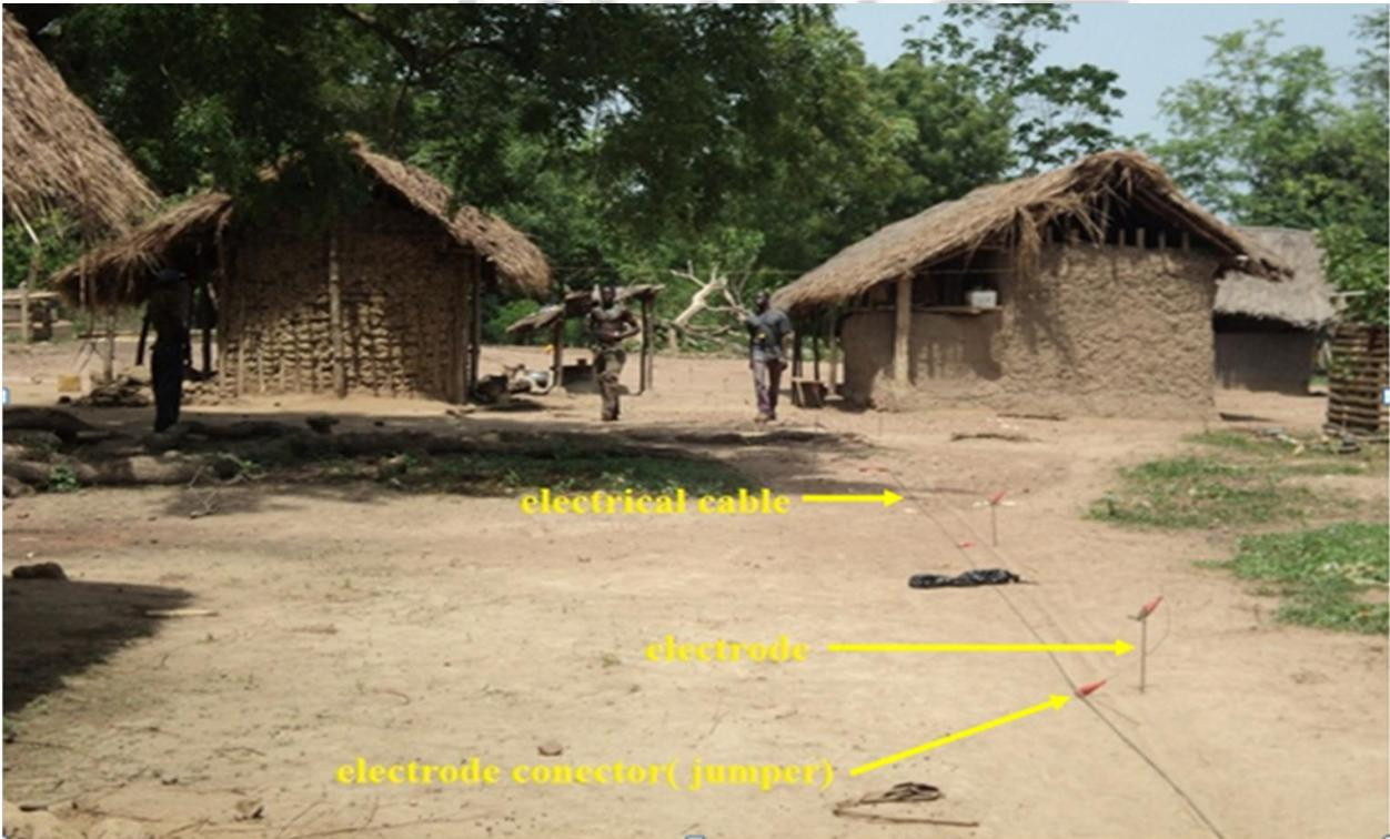
Figure 3.1 Profile line with jumpers connecting cable take-outs to steel electrodes
