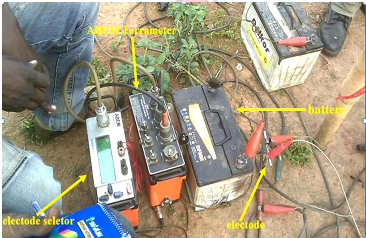
Figure 3.2 Set up of The ABEM LUND resistivity imaging equipment
