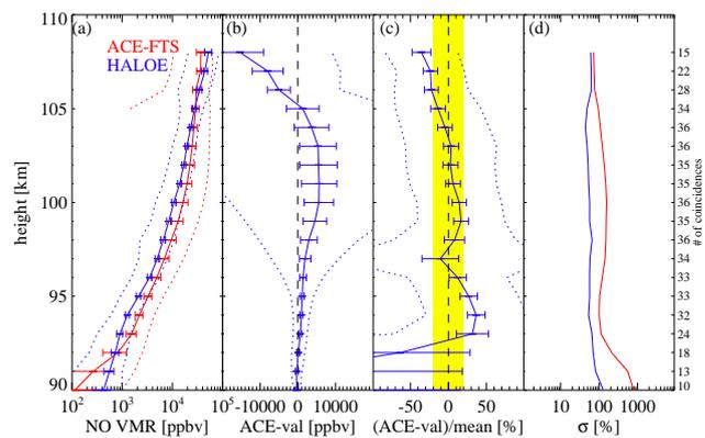
**Fig. 37.** Same as Fig. 36 but for the height range 90 to 108 km and with logarithmic abscissae for panel (a) and (d). One of the standard deviation curves in panel (a) is discontinuous because of the logarithmic axis.
