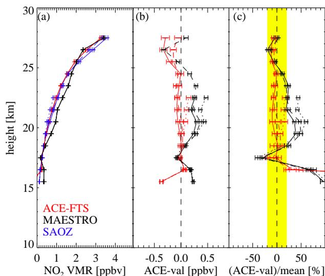
**Fig. 25.** (a) NO<sub>2</sub> profiles obtained by SAOZ at Niamey, Niger on 7 (dotted blue), 10 (solid blue) and 19 August 2006 (dashed blue); ACE occultation sunset 16076 on 7 August 2006, ACE-FTS in red and MAESTRO in black. (b) Absolute differences between SAOZ and the ACE instruments. (c) Relative differences between SAOZ and the ACE instruments. The region  $\pm 20\%$  is highlighted in yellow. Error bars represent the combined random error for panels (b) and (c).
