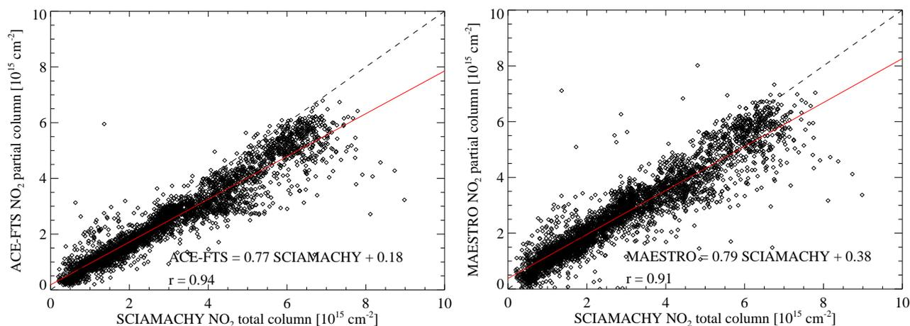
**Fig. 22.** Scatter plot of the ACE-FTS (left) and the MAESTRO (right) NO<sub>2</sub> partial columns (calculated between 14.5 to 46.5 km) and the SCIAMACHY NO<sub>2</sub> nadir total columns. In both figures the red lines are the least-squares linear fit to the data, with the slope, intercept, and correlation coefficient given in the figures. The dashed black lines show the one-to-one line relationship for comparison.
