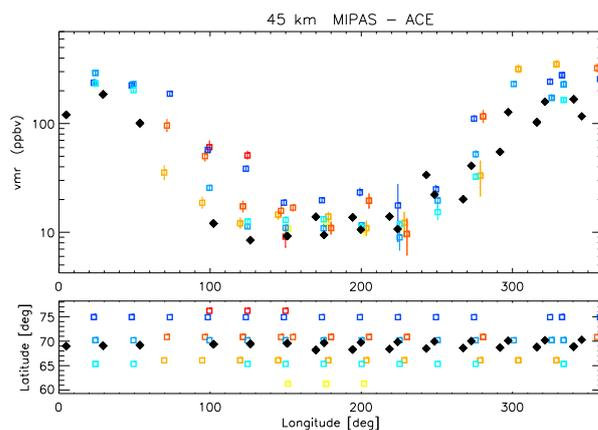
**Fig. 32.** Longitudinal distributions of ACE-FTS and MIPAS IMK-IAA NO<sub>x</sub> abundances measured on 18 March 2004 at VMR peak height (top) and respective geographic locations of the measurements (bottom). The error bars indicate random errors. Black diamonds: ACE-FTS, open squares: MIPAS (color coding: yellow, orange, red: daytime measurements; green, blue: nighttime measurements).
