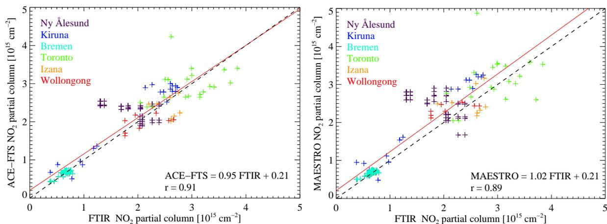
**Fig. 26.** Scatter plots of the ACE-FTS (left) and the MAESTRO (right) and ground-based FTIR NO<sub>2</sub> partial columns. For both panels the red lines are the linear least-squares fit to the data, with the slope, intercept, and correlation coefficient given in the figures. The black lines show the one-to-one linear relationship for comparison.
