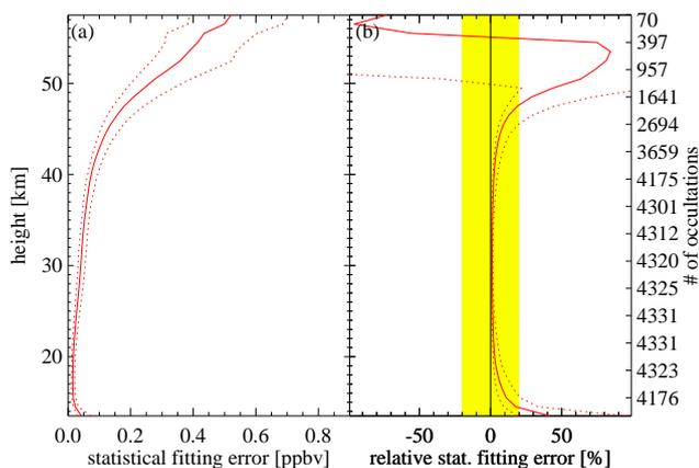
**Fig. 3.** ACE-FTS statistical fitting errors for NO<sub>2</sub> using all available data from 2005. Profiles are shown for the median (solid), and 16th and 84th percentiles (dotted) of the (a) absolute and (b) relative statistical fitting errors.
