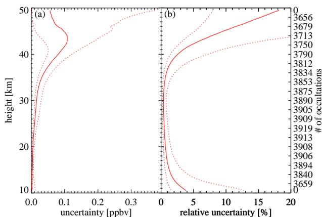
**Fig. 2.** MAESTRO uncertainties for NO<sub>2</sub> using all available data from 2005. Profiles are shown for the median (solid), and 16th and 84th percentiles (dotted) of the (a) absolute and (b) relative uncertainties.
