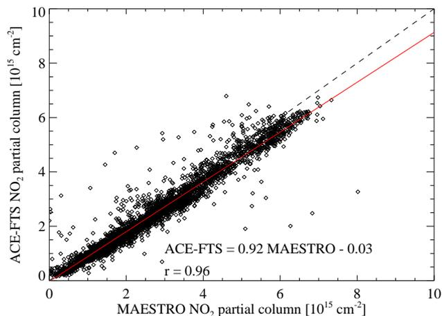
**Fig. 8.** Scatter plot of the ACE-FTS and the MAESTRO NO<sub>2</sub> partial columns (14.5 to 46.5 km). Data shown is used for the SCIAMACHY nadir comparisons (Sect. 5.1.6). The solid red line is the linear least-squares fit to the data, with the slope, intercept, and correlation coefficient given in the figure. The dashed black line shows the one-to-one linear relationship for comparison.
