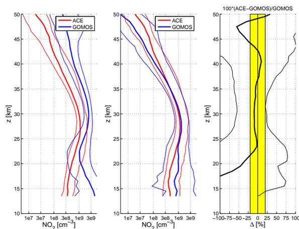
**Fig. 18.** Left: Uncorrected ACE-FTS and GOMOS weighted median profiles (thick lines) with the 16th and 84th percentiles (thin lines). Middle: Diurnal scaling has been taken into account. Right: Weighted median of the differences ( $\Delta$ ) between ACE-FTS and GOMOS. Note: the relative median difference is calculated with respect to the GOMOS median profile.
