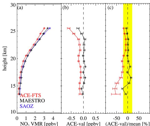
**Fig. 24.** (a) NO<sub>2</sub> profiles obtained by SAOZ at Aire-sur-l'Adour on 7 May 2005 (blue), sunrise occultation 9317 on 6 May 2005: ACE-FTS (red) and MAESTRO (black). (b) Absolute differences between SAOZ and the ACE instruments. (c) Relative differences between SAOZ and the ACE instruments. The region  $\pm 20\%$  is highlighted in yellow. Error bars represent the combined random error for panels (b) and (c).
