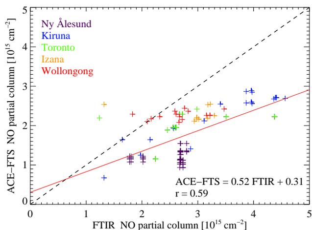
**Fig. 38.** Scatter plot of the ACE-FTS and ground-based FTIR NO partial columns. The red line is the linear least-squares fit to the data, with the slope, intercept, and correlation coefficient given in the figure. The black line shows the one-to-one line relationship for comparison.
