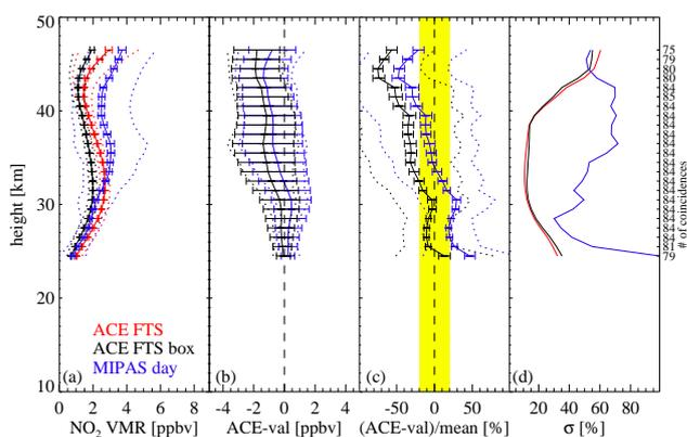
**Fig. 19.** Same as Fig. 10 but for ACE-FTS and MIPAS ESA. In addition to the ACE-FTS box model corrected data (ACE-FTS box, black), the uncorrected data is plotted (ACE-FTS, red). Note: here the error bars in panel (b) are the combined random errors.
